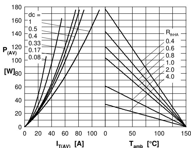
Fig. 7a Power dissipation versus direct output current
