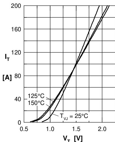
Fig. 1 Forward characteristics
