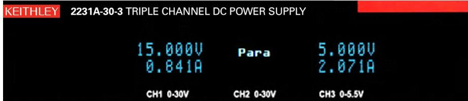
Wire the two 30V channels in series or parallel to double the output voltage to 60V or the supplied current to 6A. The Model 2231A-30-3 has series and parallel modes that manage the channels and display the total output. This display shows the supply's parallel mode, including the output voltage and the total current from the channels wired in parallel.
