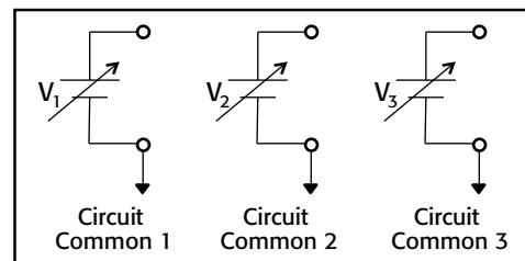
The Model 2231A-30-3 has three fully independent, programmable outputs that are electrically isolated from each other. This allows them to power circuits that are on different grounds, such as optically isolated circuits.
