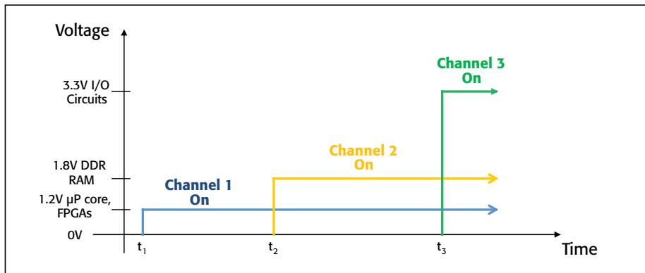
Safely power circuits up and down in the proper sequence using the three independently programmable output channels.
