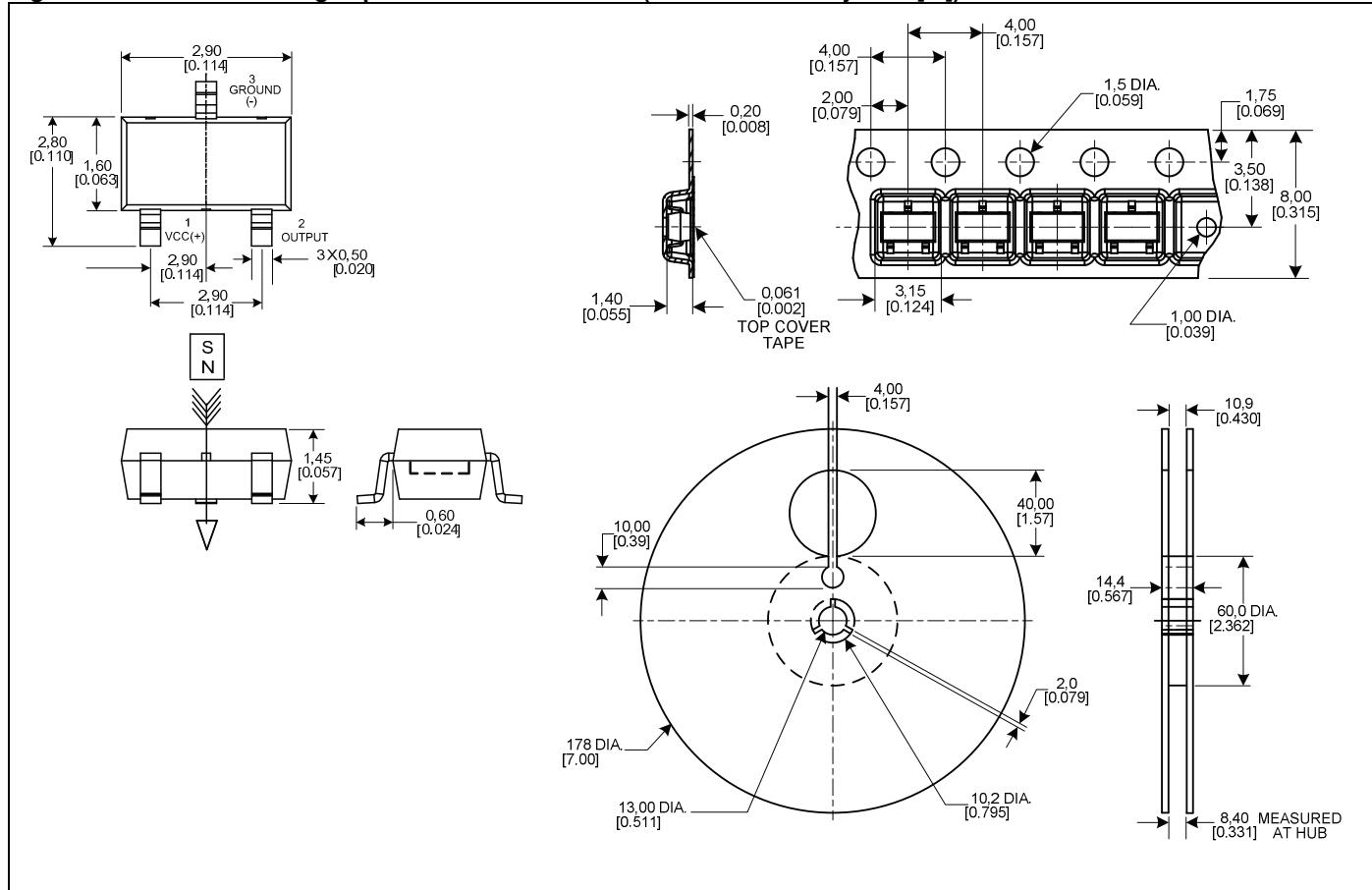
**Figure 4. SS416R Mounting Dimensions (For reference only. mm/[in])**
