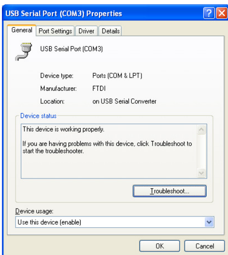
Figure 3-9 Access COM Port Properties
