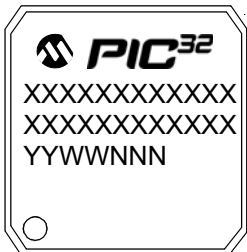
100-Lead TQFP (12x12x1 mm)
