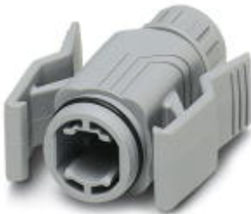
RJ45 sleeve housing, IP67, for pin insert VS-08-ST-H11-RJ45 and VS-08-ST-H21-RJ45, with push-pull interlocking for panel mounting frames, for cable cross section 5.0 mm ... 8.5 mm, color: gray
