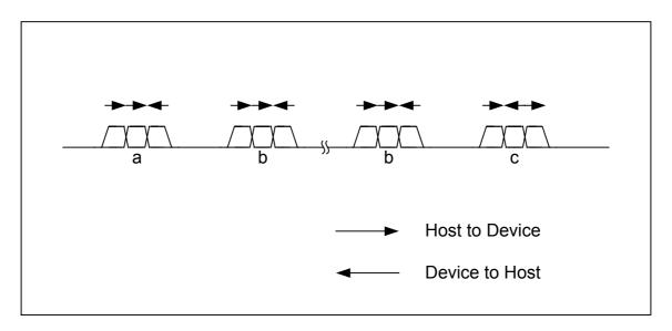
Fig. 6.29 Control transfer in host mode when the data stage is set in the OUT direction
