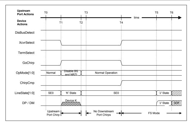
Fig. 6.12 HS Detection Handshake timing (FS mode)
