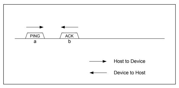
Fig. 6.25 PING transaction in host mode
