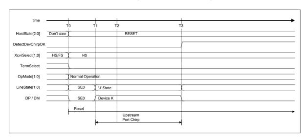
Fig. 6.41 Device chirp timing
