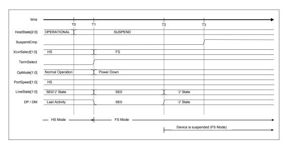
Fig. 6.55 Suspend timing (HS mode)
