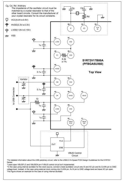
Select power supply devices carefully. The performance of such devices will affect the quality of USB signal waveforms.
