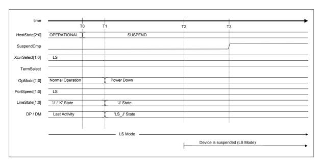
Fig. 6.57 Suspend timing (LS mode)
