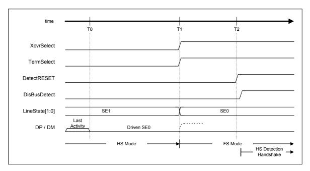
Fig. 6.10 Reset timing (HS mode)
