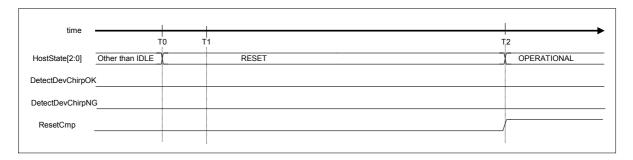
Fig. 6.65 GoRESETtoOP timing (FS or LS mode)
