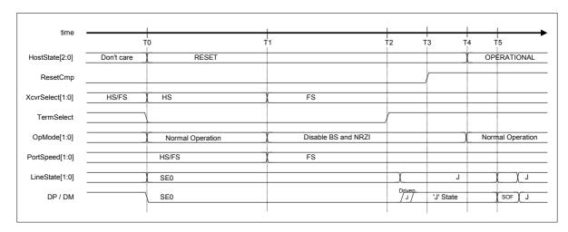
Fig. 6.52 Reset timing (FS mode)
