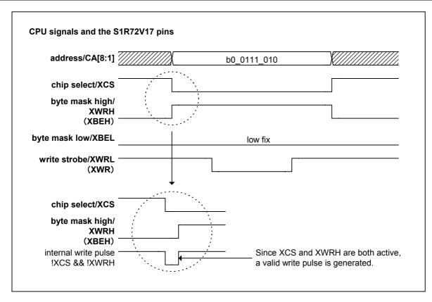
Fig. 6.71 Initializing the CPU\_Config register
