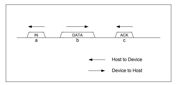
Fig. 6.3 IN transaction in device mode
