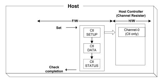
Fig. 6.31 Control by the control transfer support function
