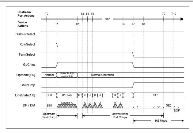
Fig. 6.13 HS Detection Handshake timing (HS mode)
