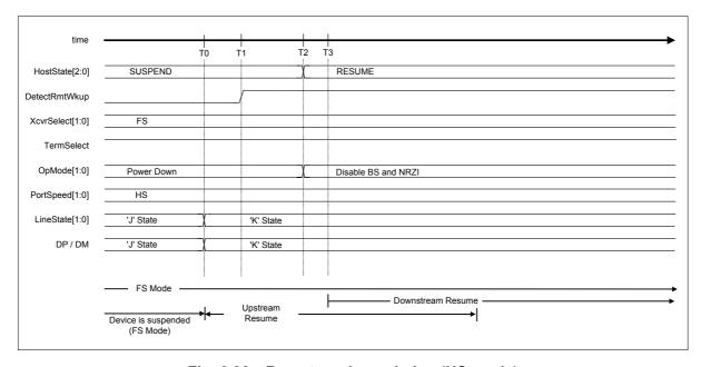
Fig. 6.38 Remote wakeup timing (HS mode)
