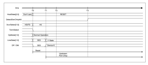
Fig. 6.42 Device chirp timing (NG)
