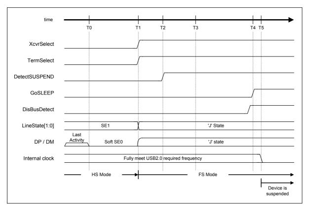
Fig. 6.8 Suspend timing (HS mode)
