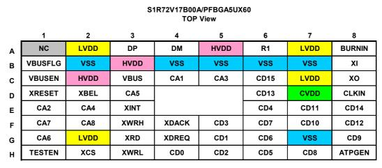
Fig. 4.1 Pin Layout Diagram of the PFBGA5UX60 package
