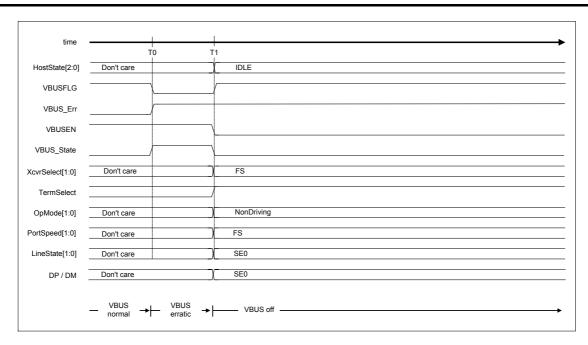
Fig. 6.35 VBUS error detection timing
