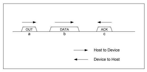
Fig. 6.23 OUT transaction in host mode
