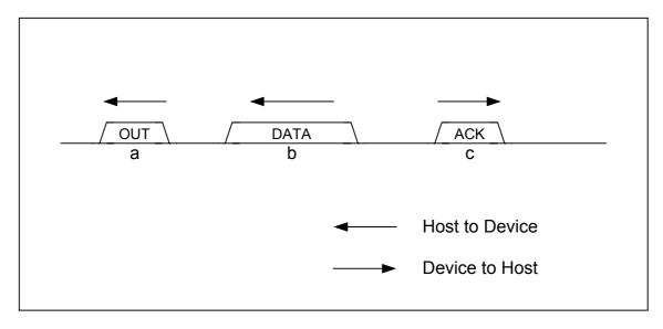
Fig. 6.2 OUT transaction in device mode
