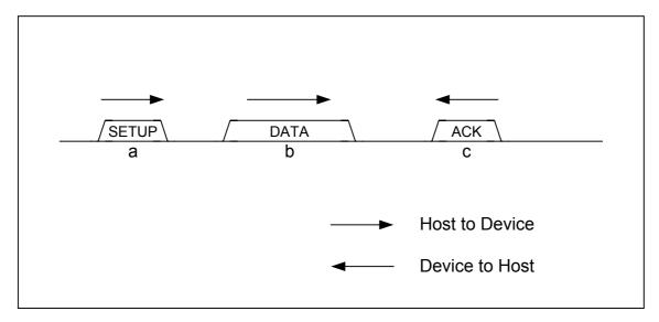
Fig. 6.22 SETUP transaction in host mode
