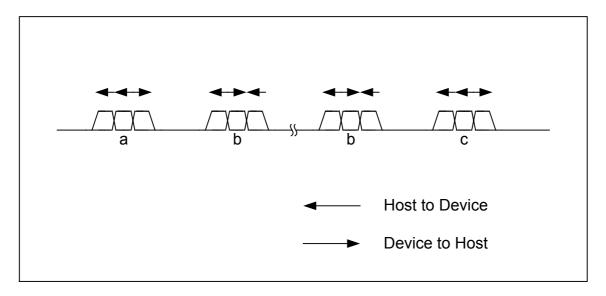
Fig. 6.6 Control transfer in device mode when the data stage is set in the IN direction
