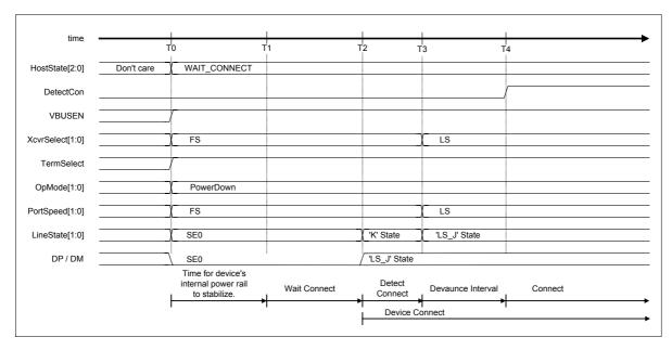
Fig. 6.45 Device attach timing (LS mode)
