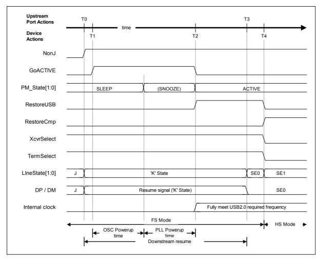
Fig. 6.16 Detect Resume timing (HS mode)
