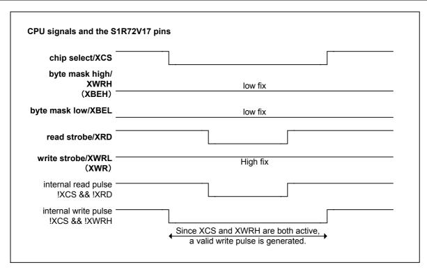
Fig. 6.72 Read access before the CPU\_Config register is initialized
