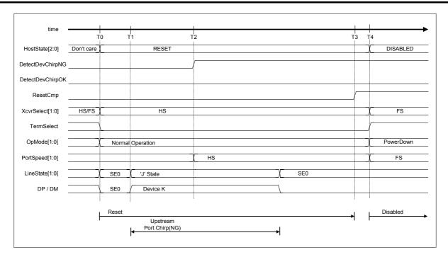
Fig. 6.50 Detect device chirp NG timing (DisChirpFinish = 0)
