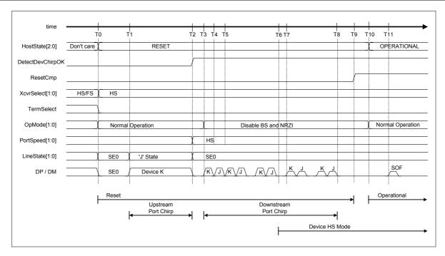
Fig. 6.49 Reset timing (HS mode)
