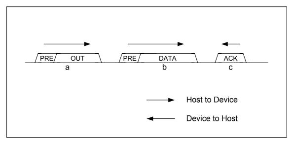
Fig. 6.26 OUT transaction with preamble attached
