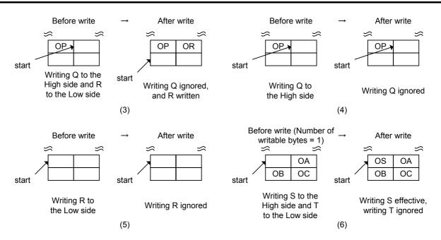
Fig. 6.73 FIFO write processing (operations that require caution)
