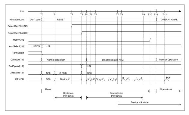
Fig. 6.51 Detect device chirp NG timing (DisChirpFinish = 1)
