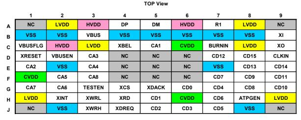
Fig. 4.2 Pin Layout Diagram of the PFBGA8UX81 package
