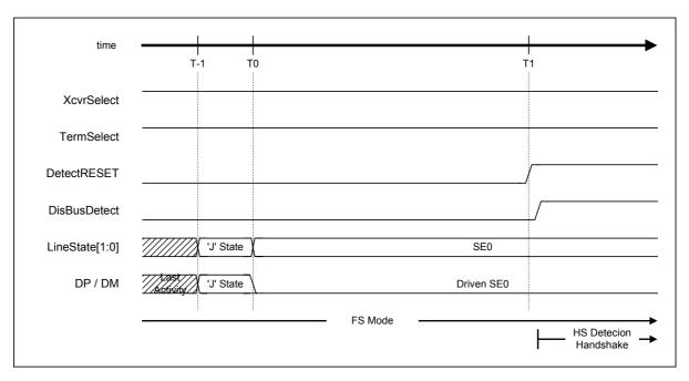
Fig. 6.11 Reset timing (FS mode)
