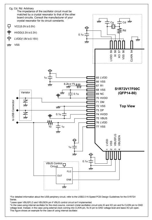
Select power supply devices carefully. The performance of such devices will affect the quality of USB signal waveforms.
