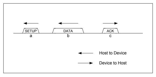
Fig. 6.1 SETUP transaction in device mode
