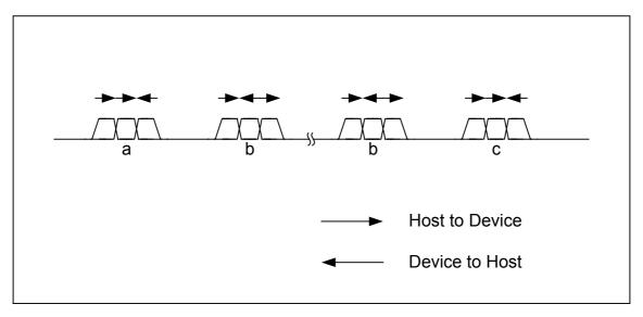
Fig. 6.30 Control transfer in host mode when the data stage is set in the IN direction
