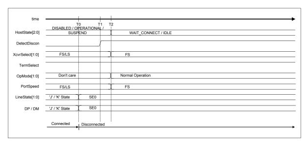
Fig. 6.37 Disconnection detection timing (FS or LS mode)
