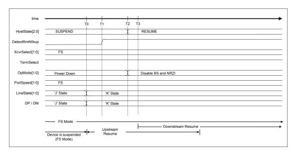
Fig. 6.39 Remote wakeup timing (FS mode)
