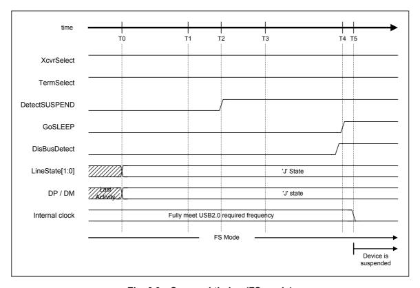
Fig. 6.9 Suspend timing (FS mode)
