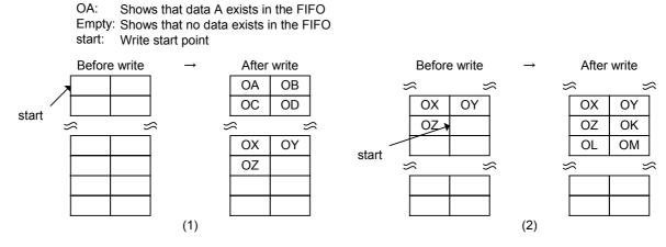
Fig. 6.72 FIFO write processing (normal operations)
