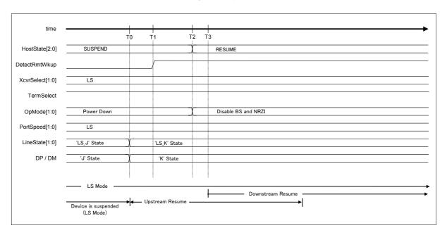
Fig. 6.40 Remote wakeup timing (LS mode)
