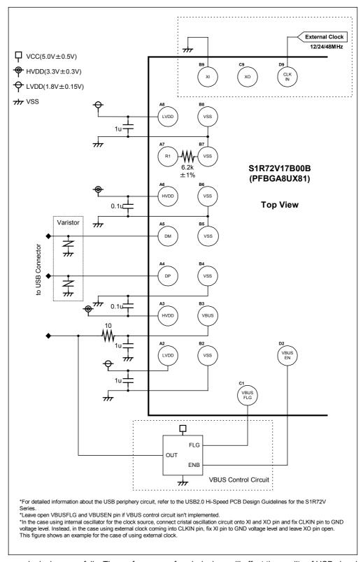
Select power supply devices carefully. The performance of such devices will affect the quality of USB signal waveforms.
