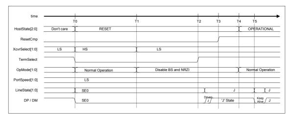
Fig. 6.53 Reset timing (LS mode)
