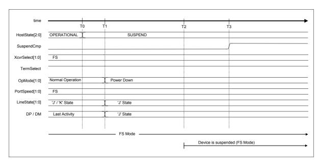
Fig. 6.56 Suspend timing (FS mode)
