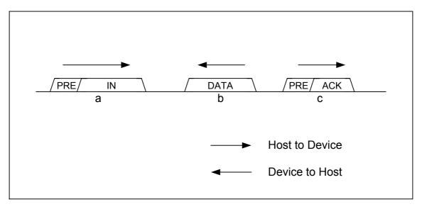
Fig. 6.27 IN transaction with preamble attached
