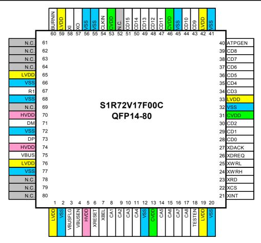
Fig. 4.3 Pin Layout Diagram of the QFP14.80 package
