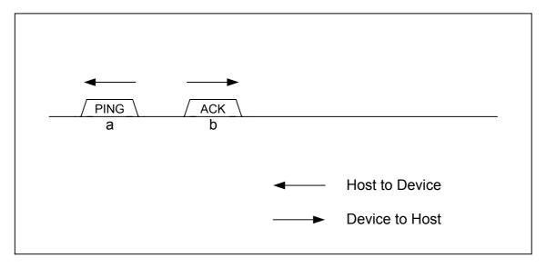
Fig. 6.4 PING transaction in device mode
