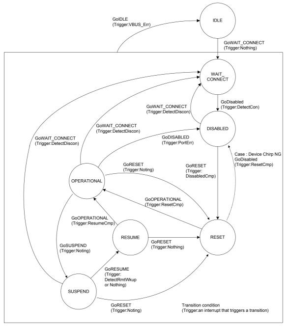
Fig. 6.34 Host state transition diagram
