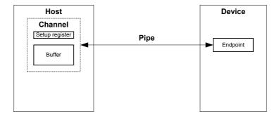
Fig. 6.18 Conceptual diagram of a channel
