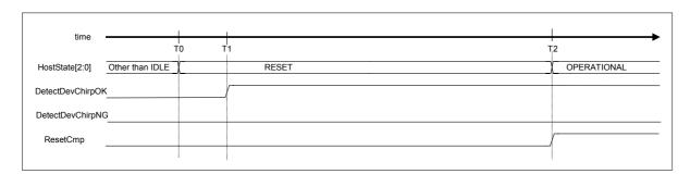
Fig. 6.64 GoRESETtoOP timing (HS mode)
