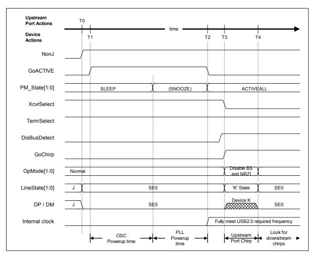
Fig. 6.14 HS Detection Handshake Timing from Suspend
