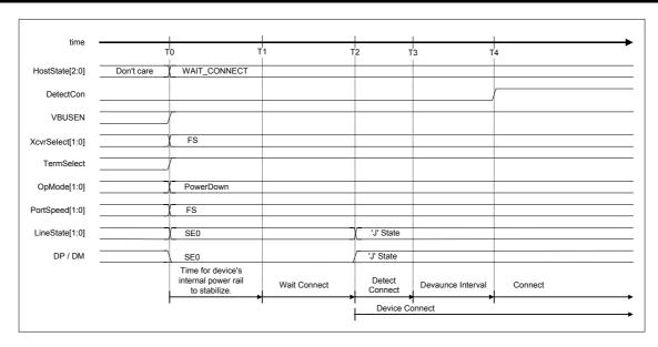
Fig. 6.44 Device attach timing (FS mode)
