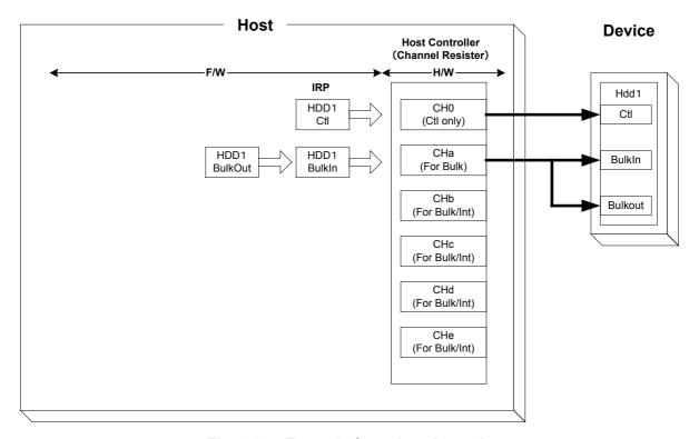
Fig. 6.20 Example for using channels (when the system has one storage device connected)
