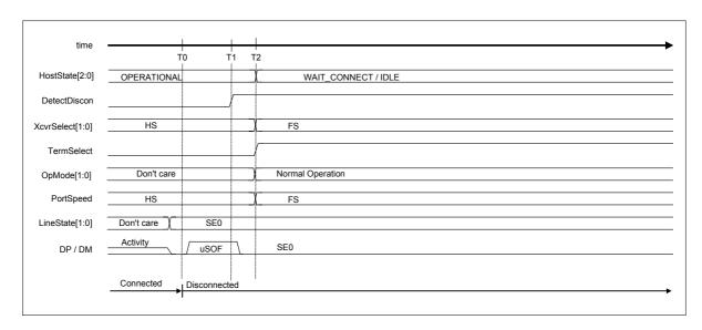
Fig. 6.36 Disconnection detection timing (HS mode)
