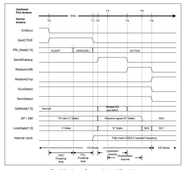
Fig. 6.15 Assert Resume timing (HS mode)
