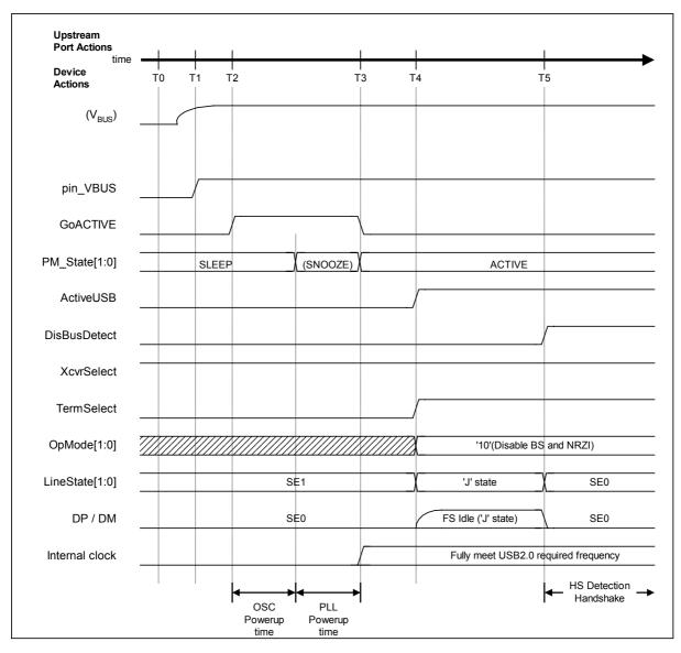
Fig. 6.17 Device Attach timing
