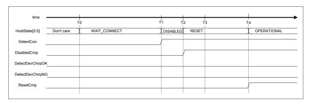
Fig. 6.63 GoWAIT\_CONNECTtoOP timing (FS or LS mode)
