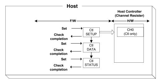
Fig. 6.28 Controlling a control transfer
