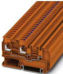
Sensor/actuator terminal block, Connection method: Push-in connection, Cross section: 0.2 mm 2 - 4 mm 2 , AWG: 24 - 12, Width: 7 mm, Color: orange, Mounting type: NS 35/7,5, NS 35/15
