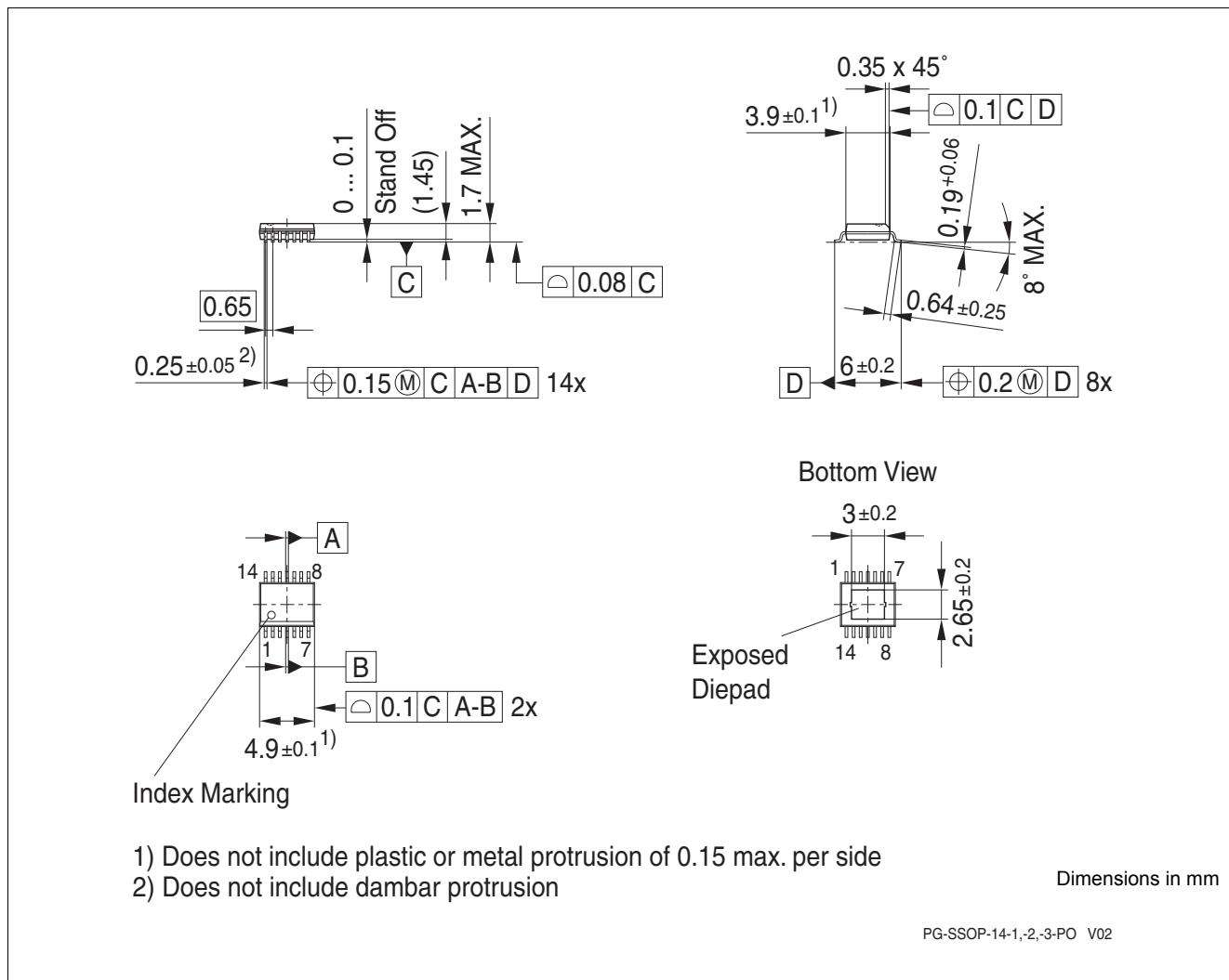
Figure 13 PG-SSOP-14
