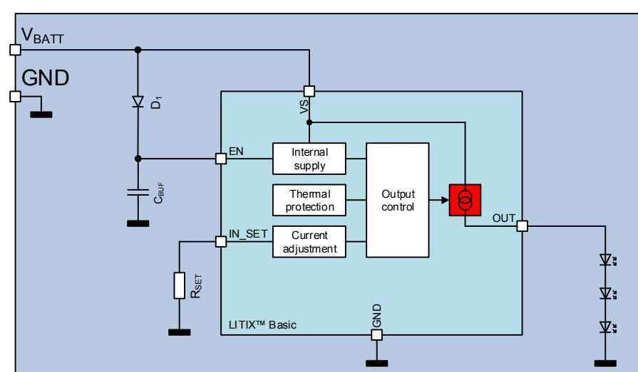
**Figure 5 External circuit when applying a fast PWM signal on  $V_{BATT}$**
