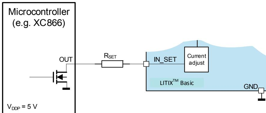
**Figure 8 Schematics IN\_SET interface to µC**
