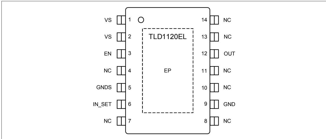
Figure 2 Pin Configuration
