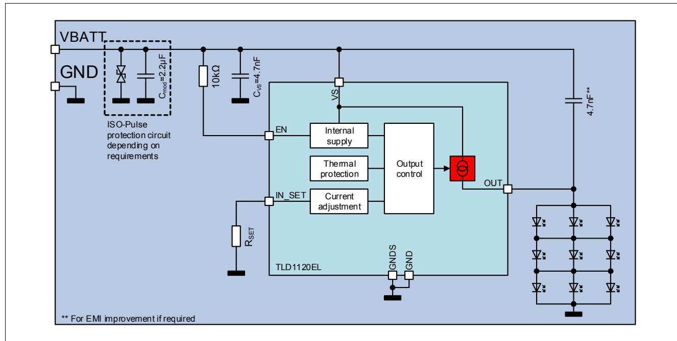
**Figure 12 Application Diagram**
