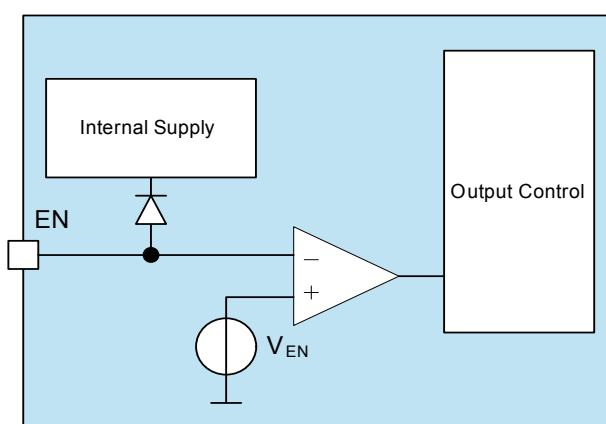
**Figure 3 Block Diagram EN pin**
