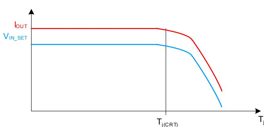
**Figure 11 Output current reduction at high temperature**
