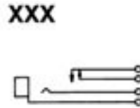
Single open circuit—“make” before “break”. (J11).
