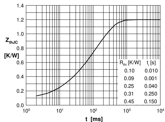
Fig. 7b Transient thermal impedance junction to case
