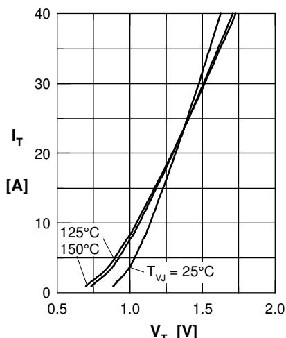
Fig. 1 Forward characteristics
