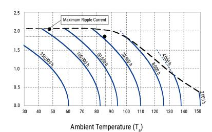
Axial Aluminum Electrolytic Capacitors - PEG126, +150°C
