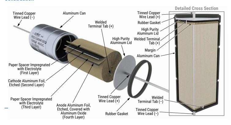
Axial Aluminum Electrolytic Capacitors - PEG126, +150°C
