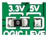
RF Meter click has an SMD jumper (zero ohm resistor) for setting the logic level either at 3.3V or 5V.
