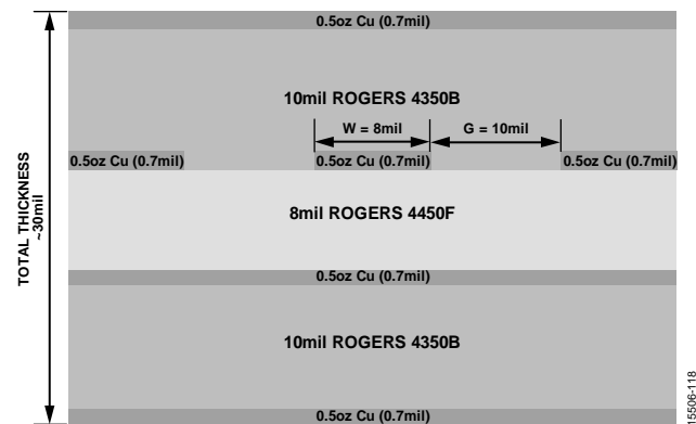
Figure 19. Evaluation Board Cross Sectional View
