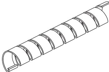
Spiral Wrap is an ideal covering used to bundle and protect tubing, wires, and other types of conductors. Spiral wrap can be used on virtually any item with a diameter of 1/16" to 7". Polyethylene Natural Spiral Wrap is a lightweight low cost material that is good for general indoor applications. Polyethylene is not affected by ordinary solvents and is resistant to abrasion.
