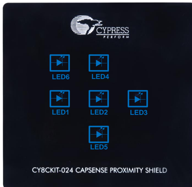
Figure 2-14: LEDs on CY8CKIT-024
