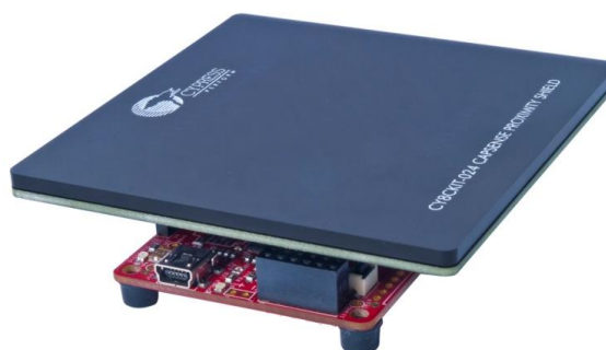
Figure 1-3: CY8CKIT-024 Connected to CY8CKIT-042
