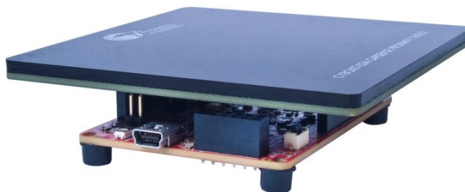
Figure 1-3: CY8CKIT-024 Connected to CY8CKIT-042
