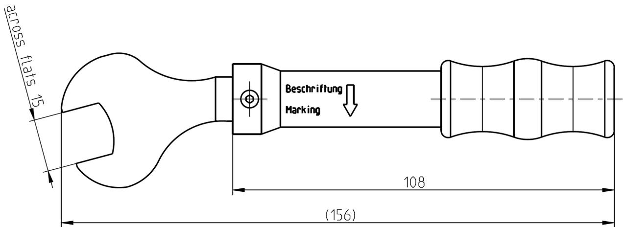
All dimensions are in mm; tolerances according to ISO 2768 m-H
