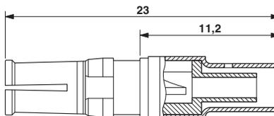
D-SUB coaxial contact pin
