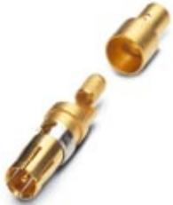
Coaxial contact, for D-SUB combination inserts, solder cup, pin, straight, for cable RG 174, gold-plated
