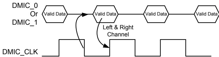
Figure 4. Stereo Digital Microphone Configuration
