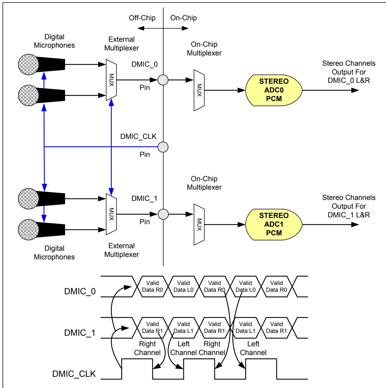
*Note: Some Digital Microphone Implementations support data on either edge, in this case the external multiplexer isn't required.*
