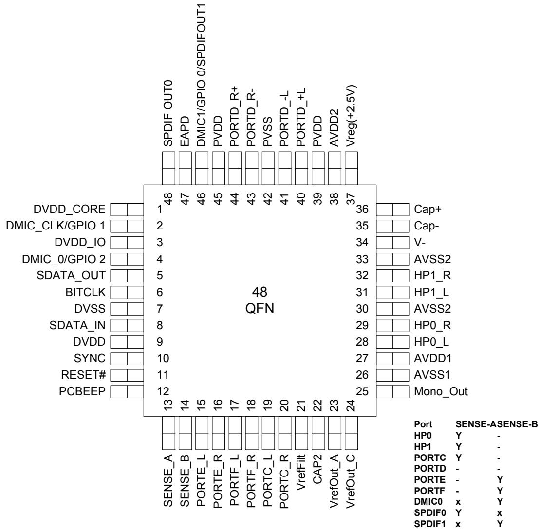
Figure 12. Pin Assignment
