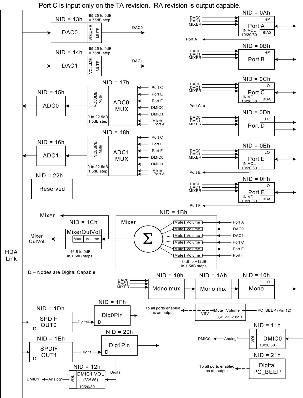
Figure 9. Widget Diagram
