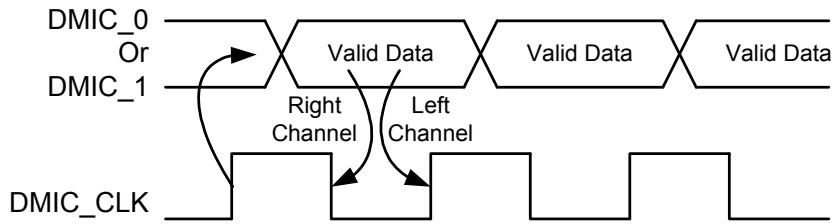
**Single “Left” Microphone, DMIC input set to mono input mode.**
