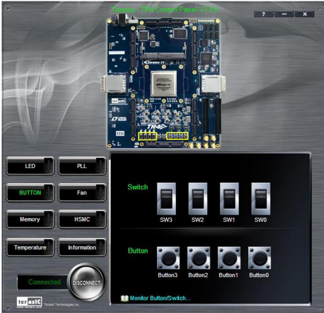
Figure 3-6 Monitoring Switches and Buttons
