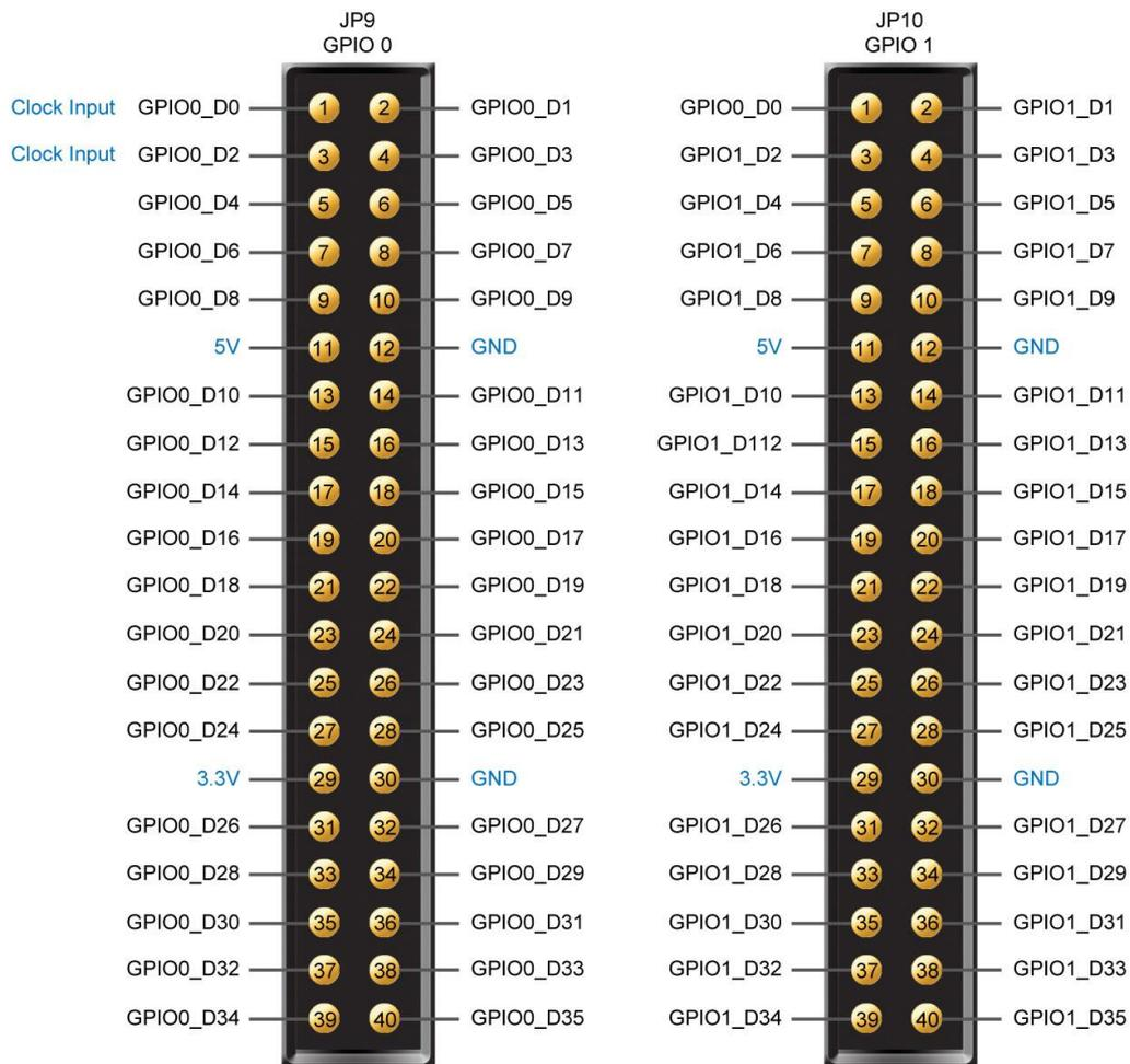
**Figure 2-21 Pin Distribution of the GPIO Expansion Headers**
