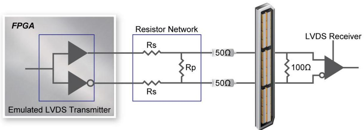
**Figure 2-12 Emulated LVDS Resistor Network between FPGA and HSMC Port**
