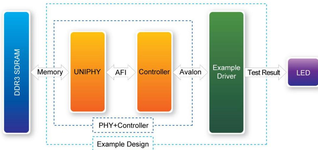
**Figure 5-9 Block Diagram of the DDR3 4G Demonstration**
