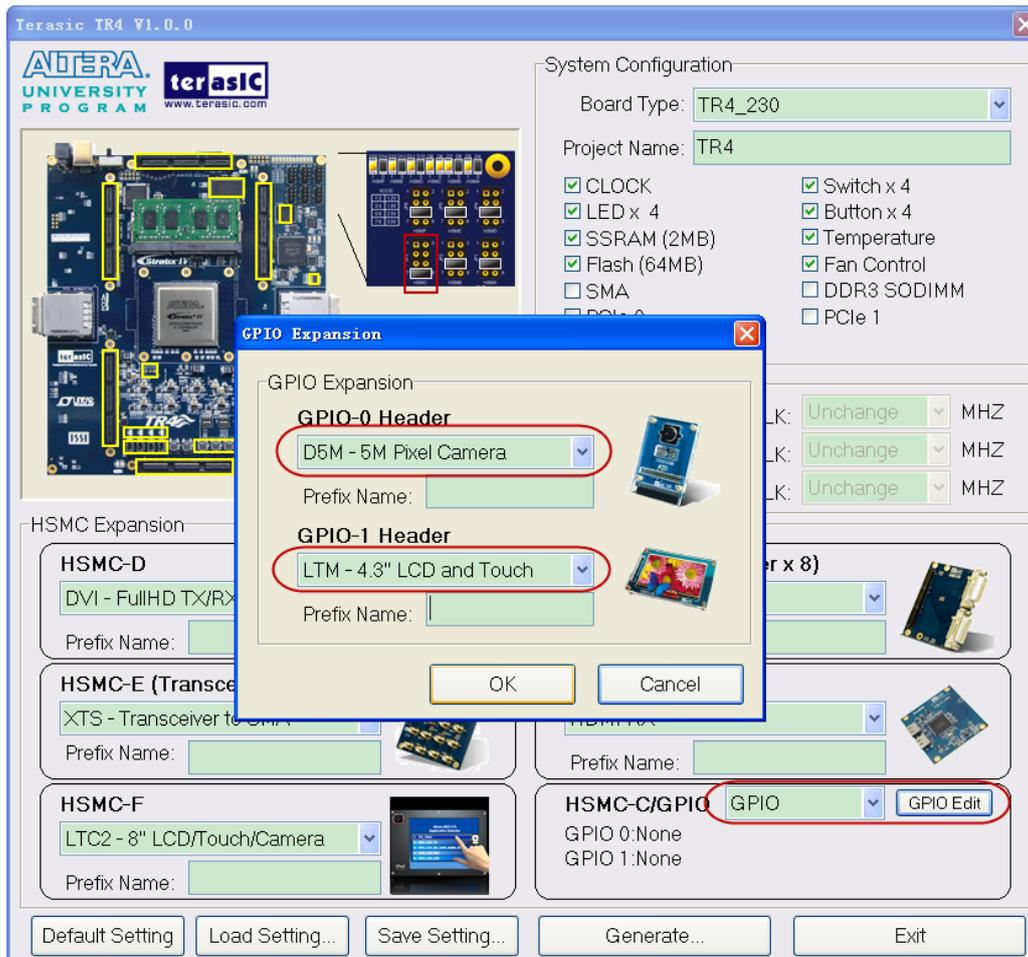
Figure 4-9 GPIO option and I/O standard recommend
