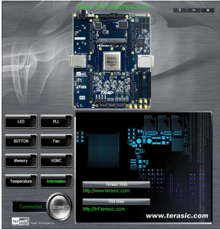
Figure 3-13 Information Tab of TR4 Control Panel
