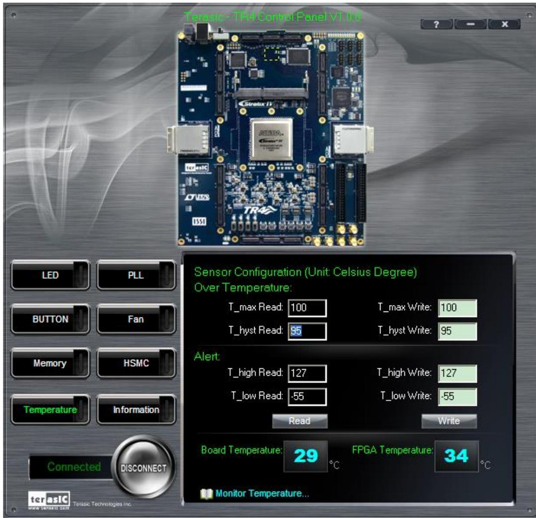
Figure 3-9 Accessing the Temperature Sensor through Control Panel
