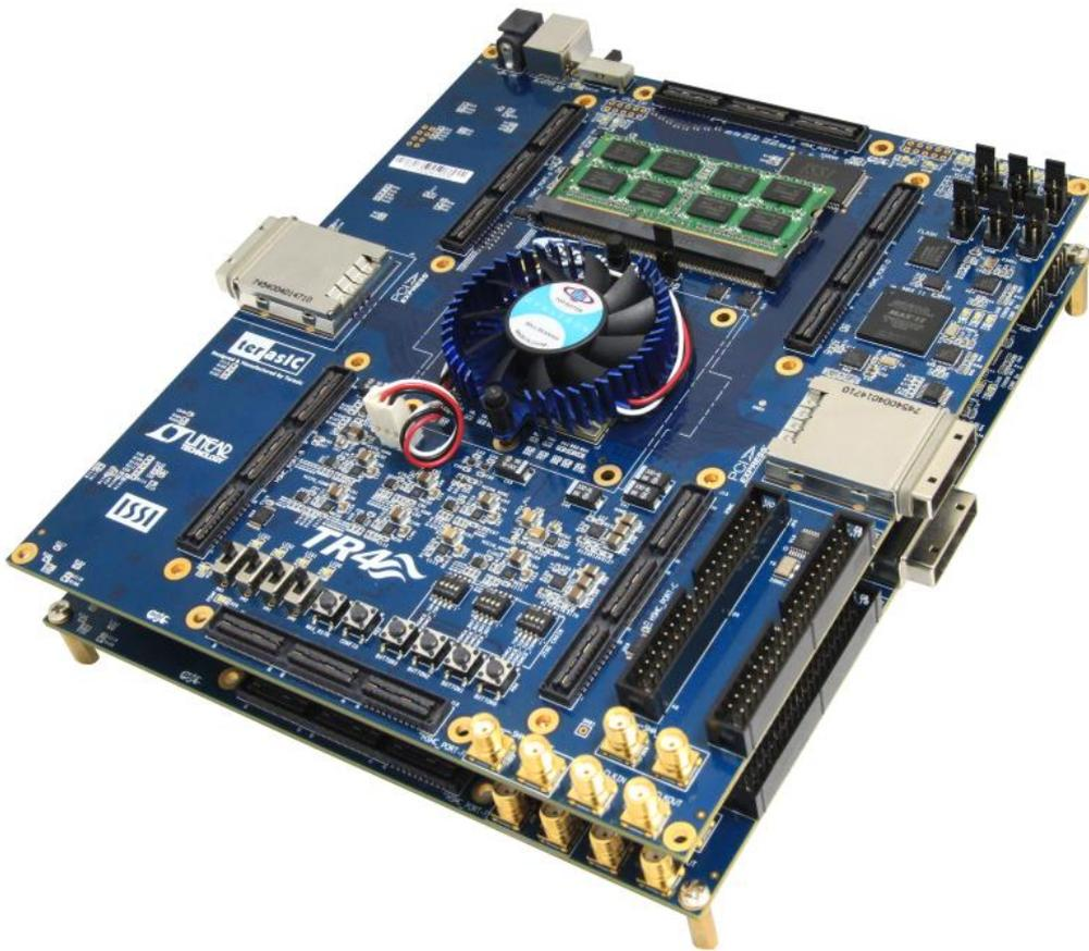
**Figure 2-19 Two Stacked TR4 Boards**
