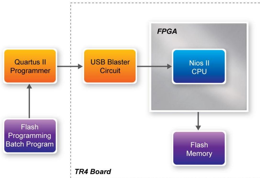
Figure 2-2 Flash Programming Scheme
