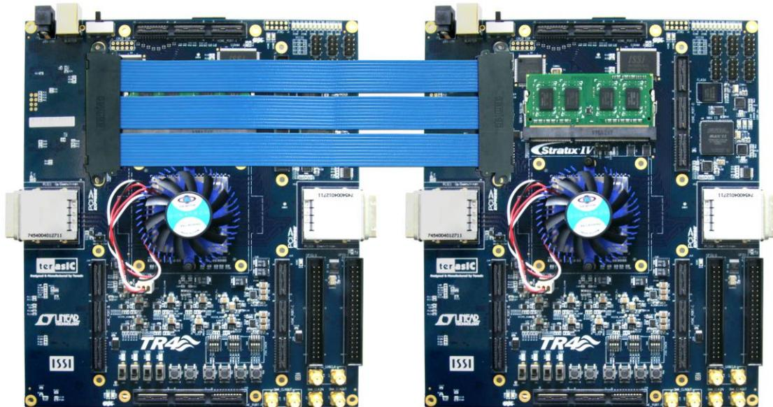
Figure 2-20 Two TR4 Boards Connected via HSMC Cable
