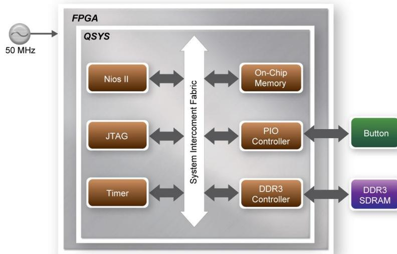
**Figure 5-6 Block diagram of the DDR3 1G demonstration**
