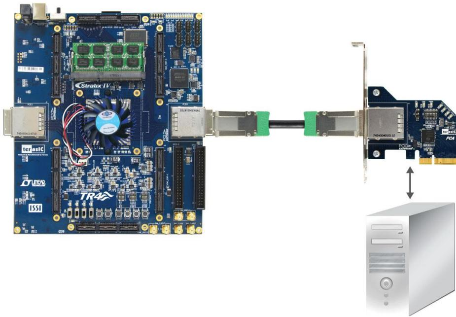
Figure 2-27 PCIe Link Setup between TR4 and PC
