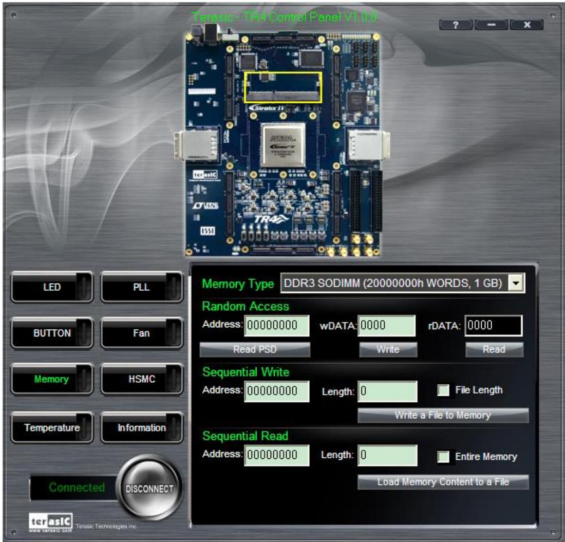
Figure 3-7 Access DDR3 SO-DIMM Memory
