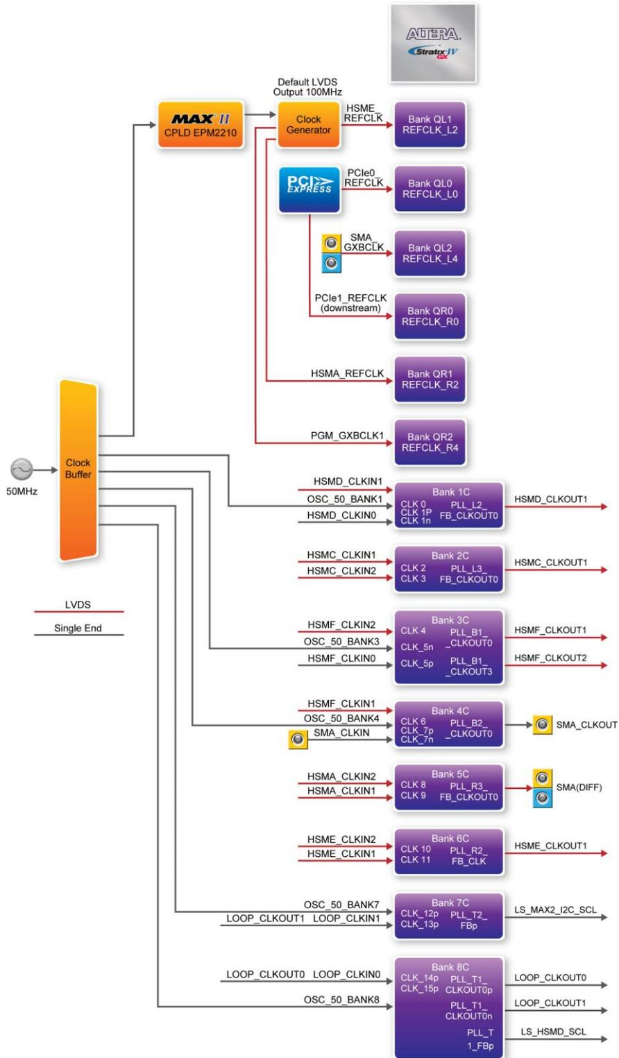
Figure 2-24 Clock Connections of the TR4
