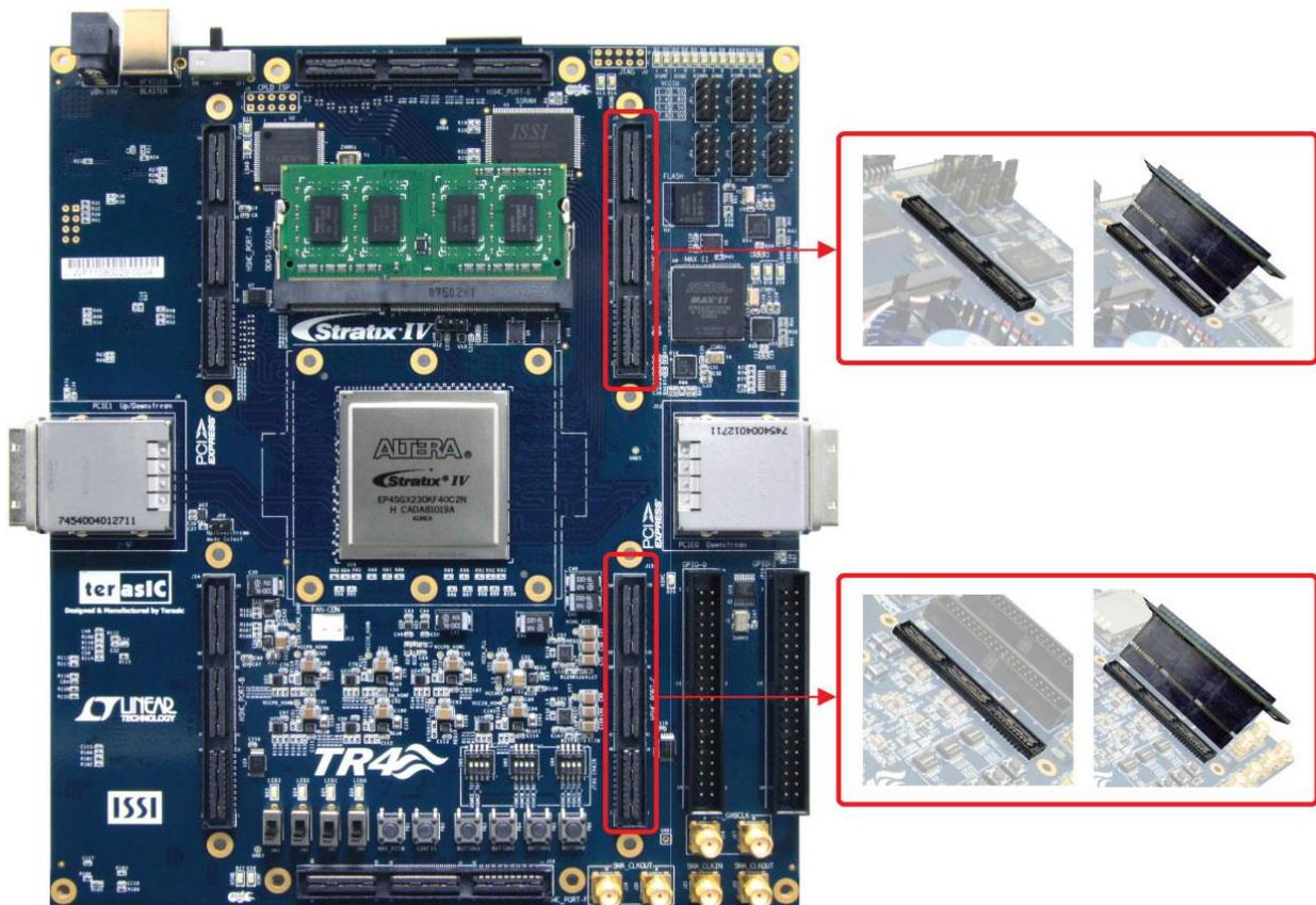
Figure 2-15 Connection between HMF2 Adapter Card and HSMC
