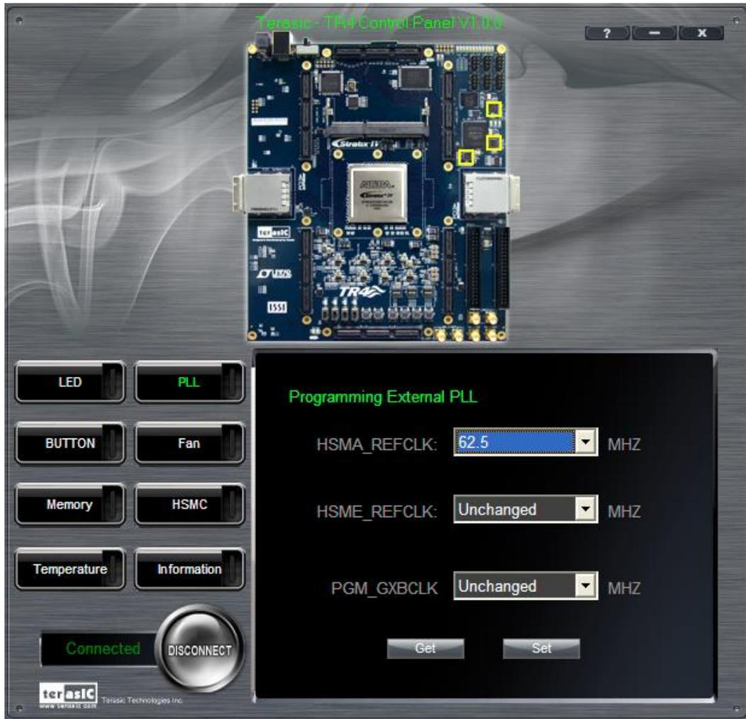
Figure 3-10 Programmable External PLL Configured through Control Panel
