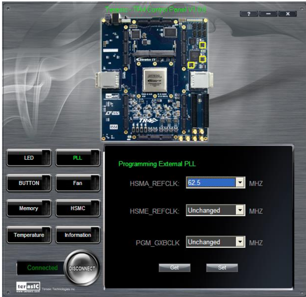
Figure 3-10 Programmable External PLL Configured through Control Panel
