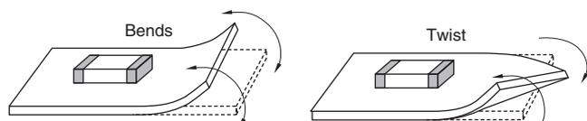
(2) During each substrate operational check, push pressure with contact failure of check pin of boards checkers of check pin may be toned up to be prevented. As substrate is bent under loading, NTC thermistor is broken owing to stress. There is also the possibility that solder on the terminal electrode will peel off. Follow the diagram for reference, and check that the substrate bends, please.
