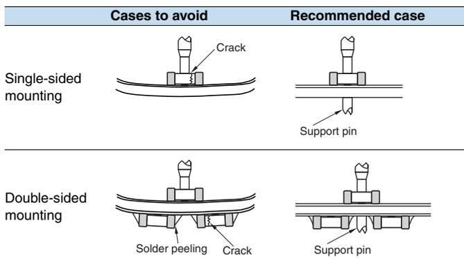
Mechanical shock that, if positioning your nail to wear, ragged edge of positionings, participates in NTC thermistor are locally, and NTC thermistor, as there is possibility of crack generated, cut the closed positioning, and maintenance and inspection, and, exchange of manage dimensions and position nail periodically, please.
