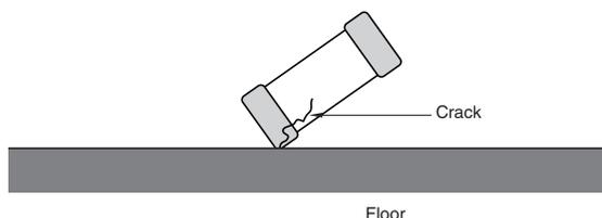
(2) At stacking storage after implementation and treatment of substrate, corner of boards is regarded as NTC thermistor. Please be careful, as there is the possibility that breakage and cracks will occur on impact.
