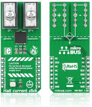
Hall current click™ is a high precision current sensor. It carries a galvanically isolated TLI4970-D050T4 miniature magnetic digital current sensor that utilizes the Hall effect to measure electric current. The board carries two EXtreme ZPower connectors to connect the conductor. The sensor readings are sent to the target board through the mikroBUS™ SPI (SDO, SCK, and CS) lines. The board uses a 3.3V power supply only.
