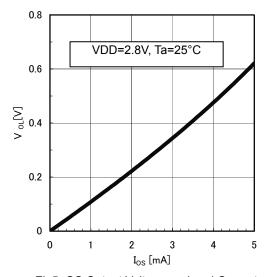
Fig5. OS Output Voltage vs. Load Current
