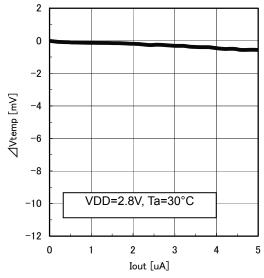
Fig4. Vtemp Voltage vs. Output Current
