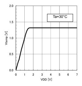
Fig2. Vtemp Voltage vs. Supply Voltage
