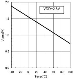
Fig3. Vtemp Voltage vs. Temperature
