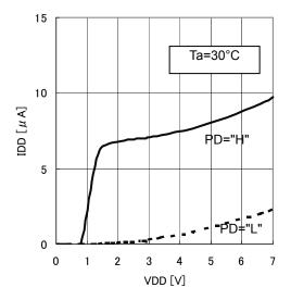
Fig1. Supply Current(IDD) vs. Supply Voltage
