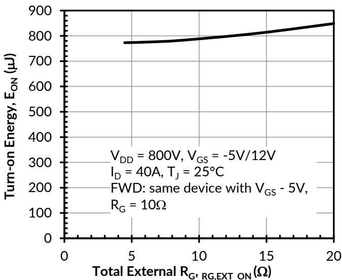
Figure 19. Clamped inductive switching turn-on energy vs.  $R_{G,EXT\_ON}$
