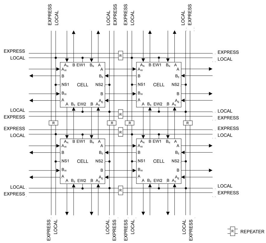
Each cell, in addition, provides the ability to route a signal on a 90° turn between the NS1 bus and EW1 bus and between the NS2 bus and EW2 bus.
