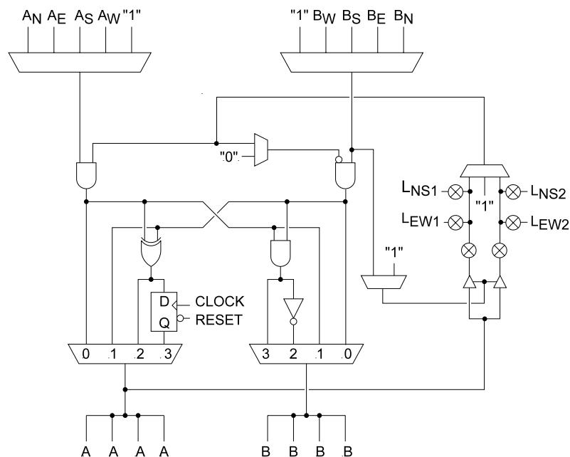
In addition to the four local-bus connections, a cell receives two inputs and provides two outputs to each of its North (N), South (S), East (E) and West (W) neighbors. These inputs and outputs are divided into two classes: "A" and "B". There is an A input and a B input from each neighboring cell and an A output and a B output driving all four neighbors. Between cells, an A output is always connected to an A input and a B output to a B input.
