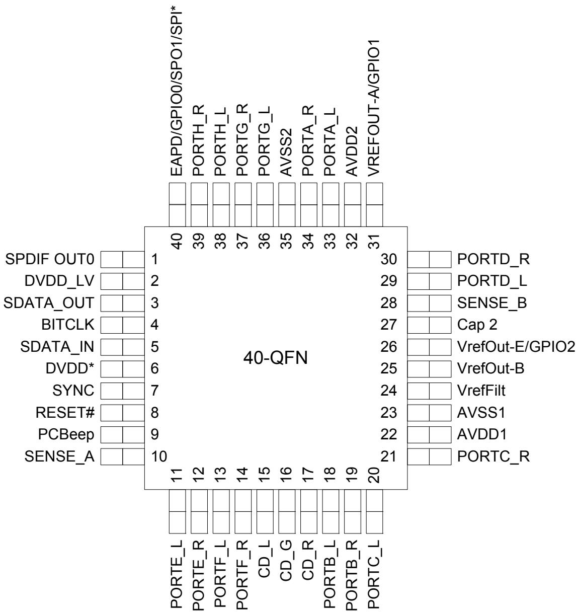
Figure 17. Pin Assignment
