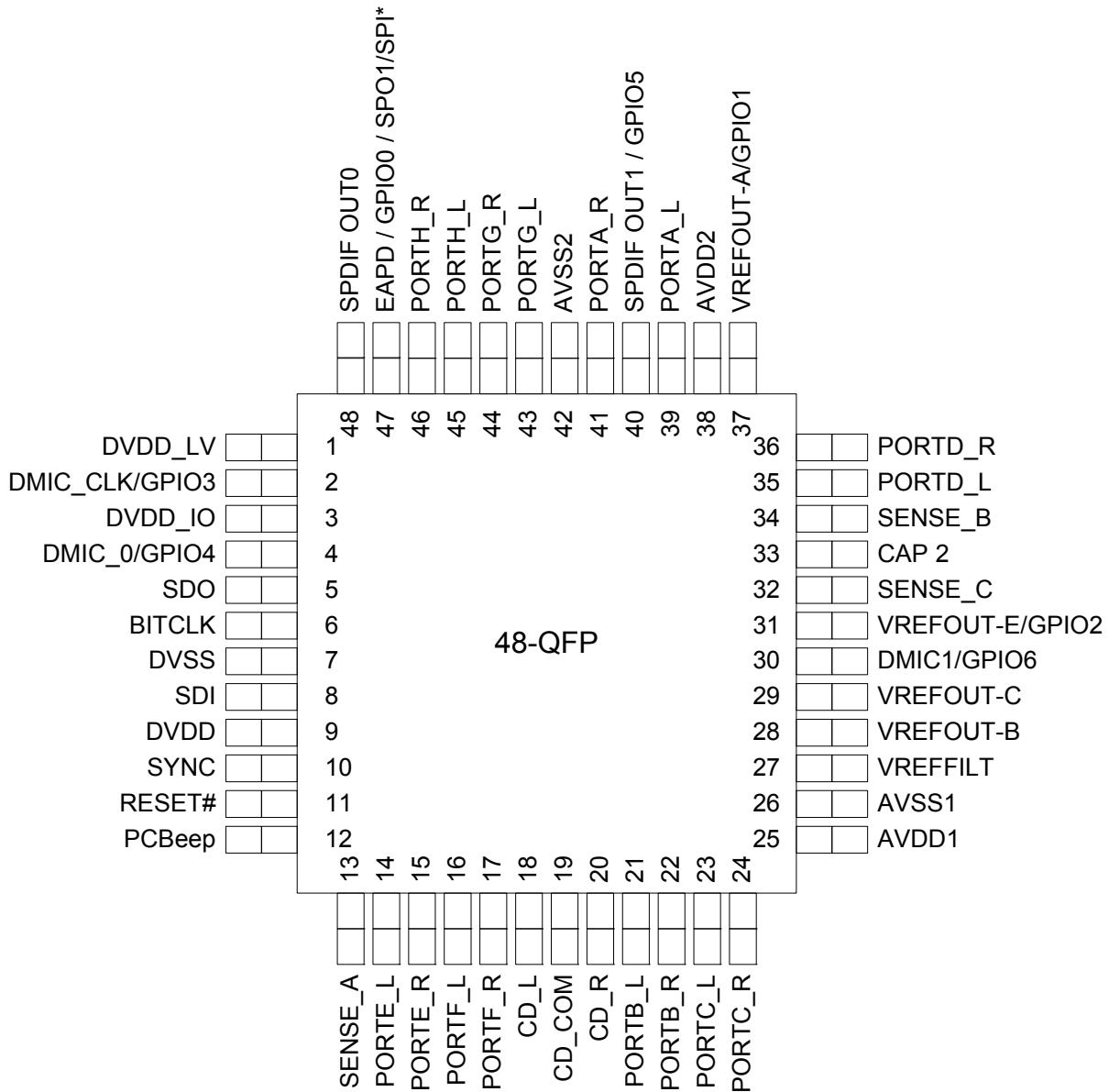
Figure 14. Pin Assignment
