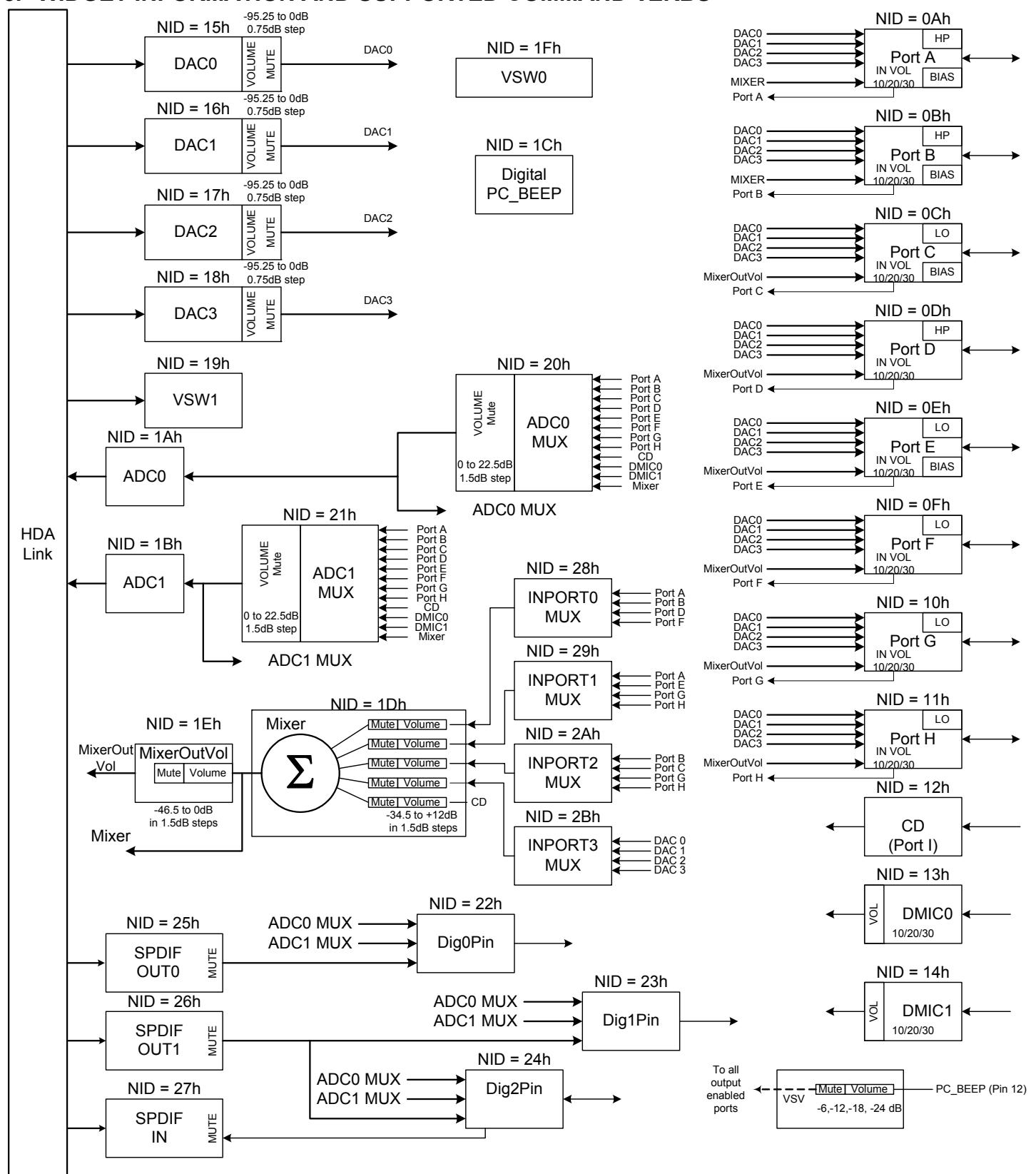
Figure 12. Widget Diagram (same for both package option)
