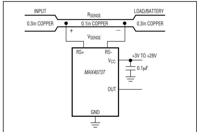
Figure 2. MAX4073T Connections Showing Use of PC Board
