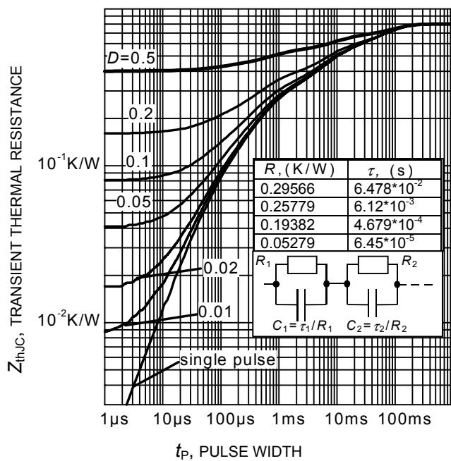
**Figure 21. IGBT transient thermal resistance**
