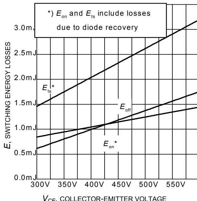
**Figure 16. Typical switching energy losses as a function of collector-emitter voltage**
