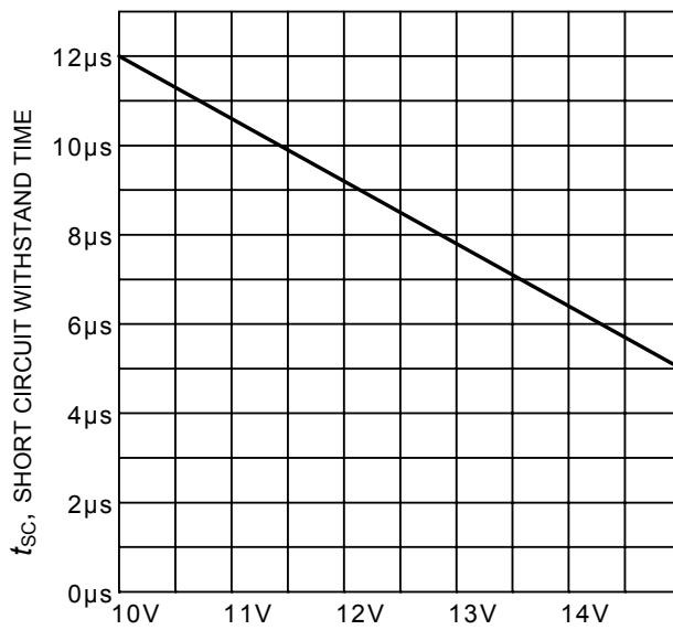
**Figure 20. Short circuit withstand time as a function of gate-emitter voltage**
