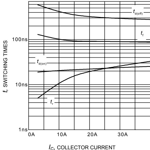
**Figure 9.** Typical switching times as a function of collector current
