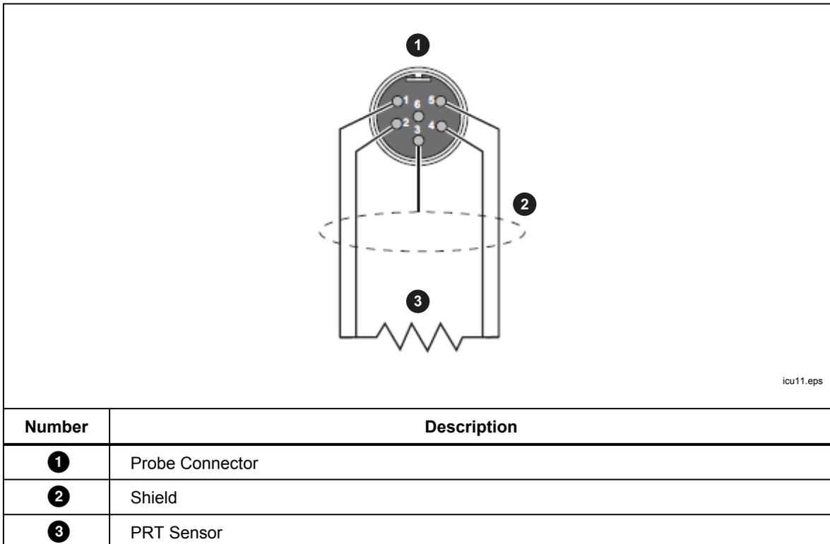
**Figure 11. Reference Probe Connections**
