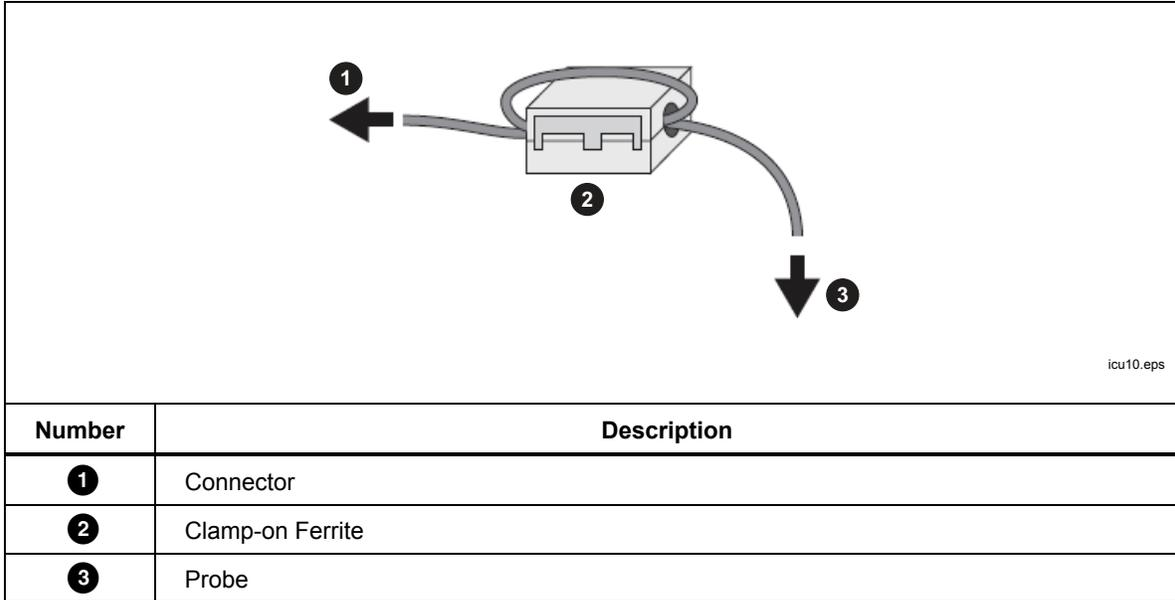
**Figure 10. Ferrite Installation**
