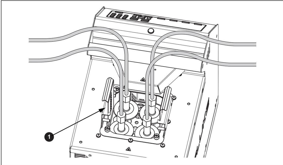
Figure 9. Adjustable Probe Fixture
