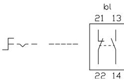
21 Selector switch actuator 2 positions 55 mm page 24 | Selector switch actuator 2 positions 70 mm page 26 | Selector switch actuator 2 positions 55 mm, flush mounting page 49 | Selector switch actuator 2 positions 70 mm, flush mounting page 51
