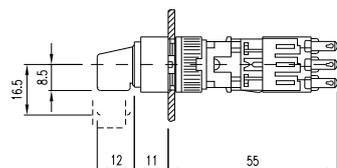
22 Keylock switch actuator 2 positions 45 mm page 17 | Keylock switch actuator 3 positions 45 mm page 22
