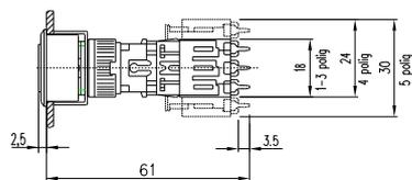
44 Illuminated pushbutton actuator 55 - 70 mm, flush mounting page 41
