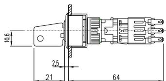
**59 Keylock switch actuator 2 positions 55 mm, flush mounting** page 43
