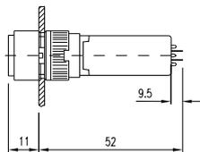
**27 Keylock switch actuator 2 positions 55 mm page 18 | Keylock switch 2 positions actuator 55 - 70 mm, momentary, switch interlock system function 2 page 33 | Keylock switch actuator 2 positions 55 mm, maintained, switch interlock system functions 1 and 3 page 35**
