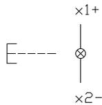
**33 Snap-action switching element block for 35 mm page 66**
