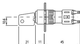
23 Selector switch actuator 2 positions 45 mm page 23 | Selector switch actuator 3 positions 45 mm page 28
