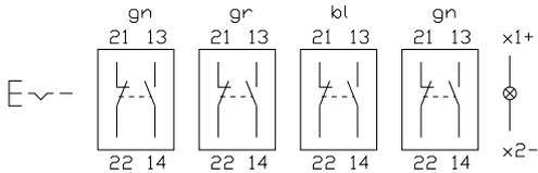
**12 Illuminated pushbutton actuator 55 - 70 mm page 12 | Illuminated pushbutton actuator 55 - 70 mm, maintained, switch interlock system variant 2 page 31 | Illuminated pushbutton actuator 55 - 70 mm, flush mounting page 41**
