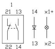
**35 Snap-action switching element block for 35 mm page 66**
