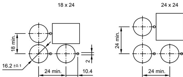
12 Buzzer actuator 30 - 55 mm, flush mounting page 40
