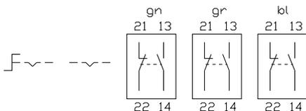
**30 Selector switch actuator 2 positions 55 mm page 24 | Selector switch actuator 2 positions 70 mm page 26 | Selector switch actuator 2 positions 55 mm, flush mounting page 49 | Selector switch actuator 2 positions 70 mm, flush mounting page 51**
