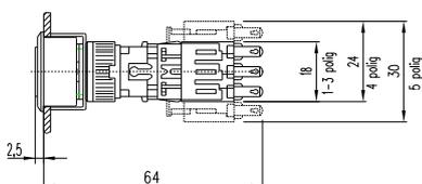
43 Illuminated pushbutton actuator 55 - 70 mm, flush mounting page 41
