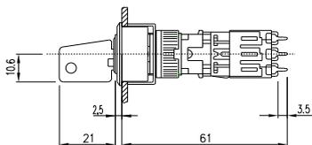
**60 Keylock switch actuator 2 positions 70 mm, flush mounting** page 45
