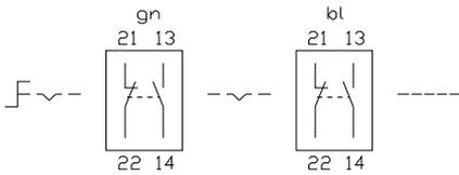
19 Selector switch actuator 3 positions 45 mm page 28 | Selector switch actuator 3 positions 45 mm, flush mounting page 53
