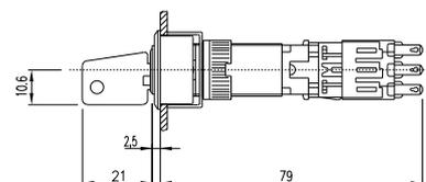
**61 Keylock switch actuator 2 positions 70 mm, flush mounting** page 45
