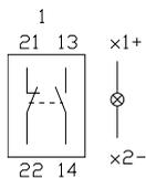
**37 Keylock switch actuator 3 positions 45 mm page 22 | Keylock switch actuator 3 positions 45 mm, flush mounting page 47**
