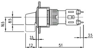
35 Selector switch actuator 2 positions 55 mm, flush mounting page 49
