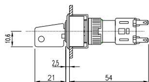
**57 Keylock switch actuator 2 positions 45 mm, flush mounting** page 42 | **Keylock switch actuator 3 positions 45 mm, flush mounting** page 47
