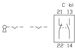
48 Keylock switch actuator 2 positions 55 mm page 18 | Keylock switch actuator 2 positions 70 mm page 20 | Keylock switch actuator 2 positions 55 mm, maintained, switch interlock system functions 1 and 3 page 35 | Keylock switch 2 positions actuator 70 mm, maintained, switch interlock system functions 1 and 3 page 37 | Keylock switch actuator 2 positions 55 mm, flush mounting page 43 | Keylock switch actuator 2 positions 70 mm, flush mounting page 45
