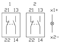
**36 Snap-action switching element block for 35 mm page 66**
