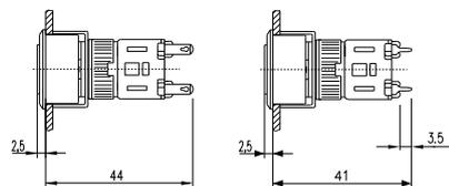
**42 Illuminated pushbutton actuator 55 - 70 mm, flush mounting page 41**
