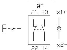
15 Illuminated pushbutton actuator 35 mm page 11 | Illuminated pushbutton actuator 35 mm, flush mounting page 40
