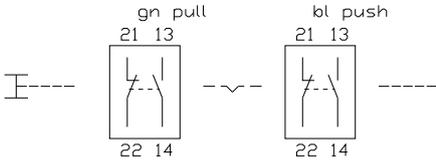
**60 Illuminated pushbutton actuator 55 - 70 mm, momentary, switch interlock system variants 1, 3 - 7 page 30 | Release button actuator 55 - 70 mm, momentary, switch interlock system variants 4 - 7 page 32**
