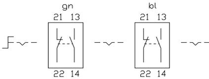
20 Selector switch actuator 2 positions 45 mm page 23 | Selector switch actuator 2 positions 45 mm, flush mounting page 48
