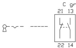
47 Keylock switch actuator 2 positions 45 mm page 17 | Keylock switch actuator 2 positions 45 mm, flush mounting page 42
