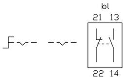
**27 Selector switch actuator 2 positions 55 mm page 24 | Selector switch actuator 2 positions 70 mm page 26 | Selector switch actuator 2 positions 55 mm, flush mounting page 49 | Selector switch actuator 2 positions 70 mm, flush mounting page 51**
