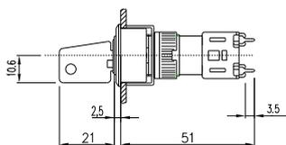
**58 Keylock switch actuator 2 positions 55 mm, flush mounting** page 43
