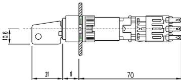
**53 Keylock switch actuator 2 positions 70 mm** page 20 | **Keylock switch 2 positions actuator 55 - 70 mm, momentary, switch interlock system function 2** page 33 | **Keylock switch 2 positions actuator 70 mm, maintained, switch interlock system functions 1 and 3** page 37
