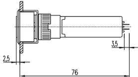
**52 Keylock switch actuator 2 positions 70 mm** page 20 | **Keylock switch 2 positions actuator 55 - 70 mm, momentary, switch interlock system function 2** page 33 | **Keylock switch 2 positions actuator 70 mm, maintained, switch interlock system functions 1 and 3** page 37
