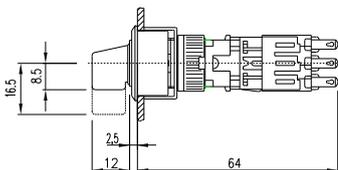
**36 Selector switch actuator 2 positions 55 mm, flush mounting page 49**
