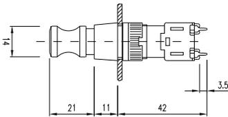
33 Selector switch actuator 2 positions 45 mm, flush mounting page 48 | Selector switch actuator 3 positions 45 mm, flush mounting page 53
