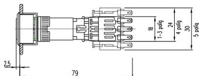
45 Illuminated pushbutton actuator 55 - 70 mm, flush mounting page 41
