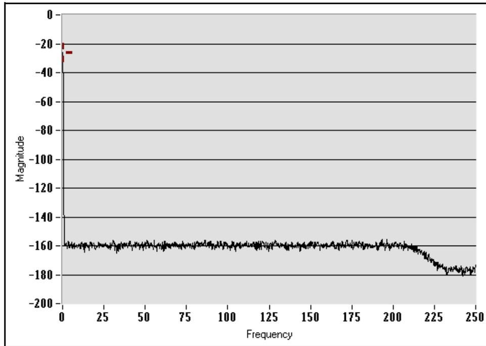
**Figure 1. Modulator Noise Performance**
