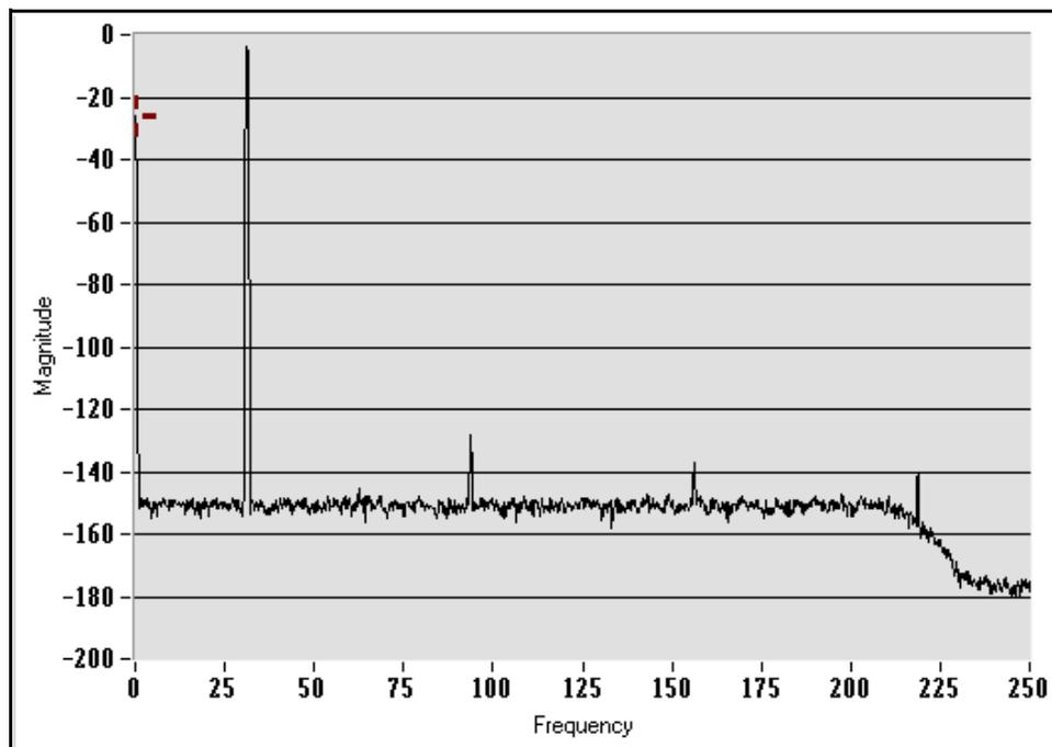
**Figure 2. Modulator + Test DAC Dynamic Performance**
