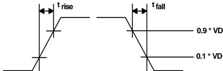
Figure 3. Digital Input Rise and Fall Times
