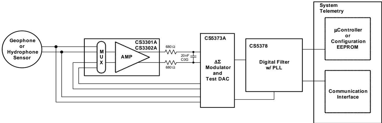
Figure 7. System Diagram
