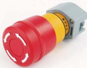
Emergency-stop, twist release, 37mm diameter, foolproof to EN 60947-5-1 and EN 418, use slow-make switching elements
