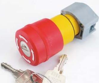
Emergency-stop, key release, 37mm diameter, foolproof to EN 60947-5-1 and EN 418, use slow-make switching elements
