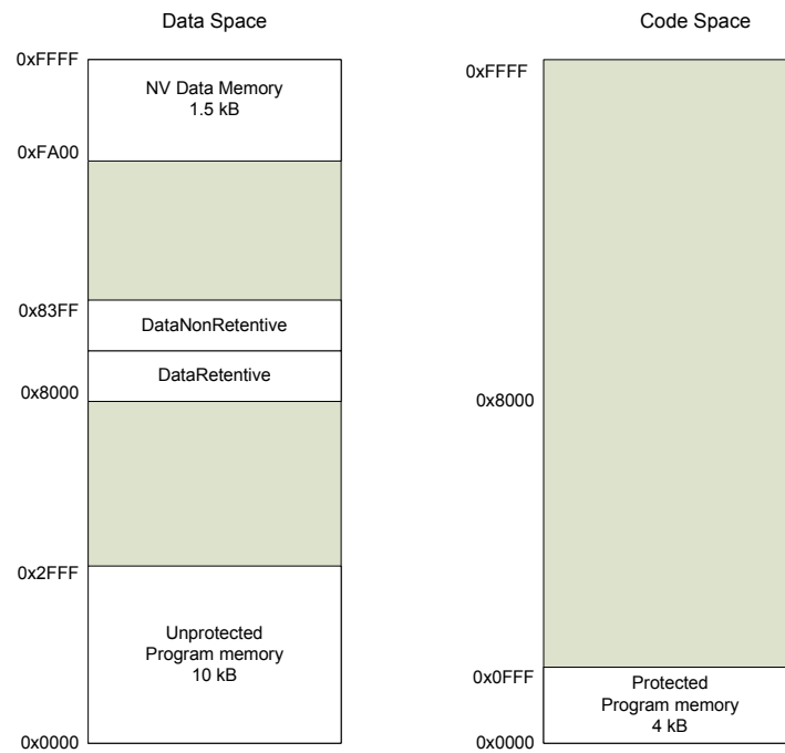
Figure 36. Example memory map with 4 kB of protected flash program memory
