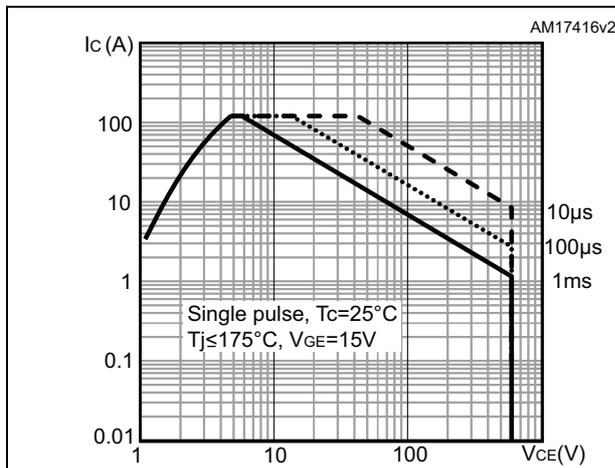
Figure 11. Safe operating area for TO-247 and TO-3P
