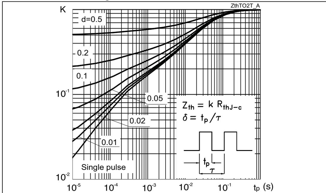
Figure 24. Thermal data for TO-3P and TO-247
