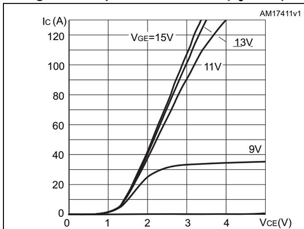
Figure 7. Output characteristics (T<sub>J</sub>=175°C)
