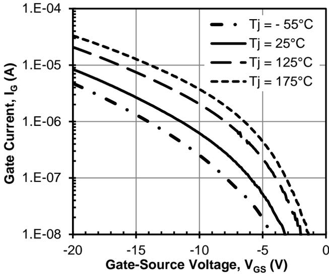
**Figure 13 Typical gate leakage current at  $V_{DS} = 0V$**
