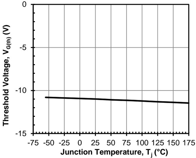
**Figure 9** Threshold voltage vs.  $T_j$
