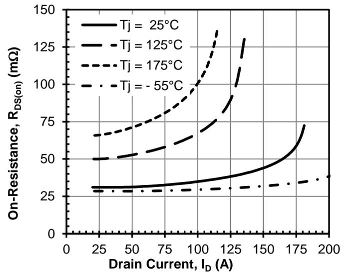
**Figure 8** Typical drain-source on-resistance at  $V_{GS} = 0V$
