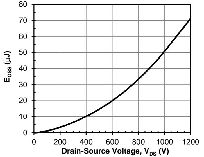
**Figure 10** Typical stored energy in  $C_{OSS}$
