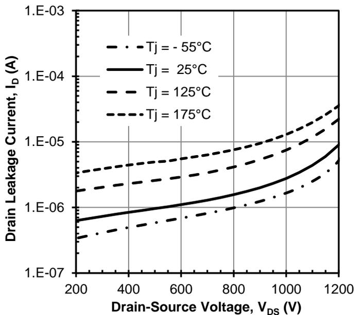
**Figure 4 Typical drain-source leakage**
