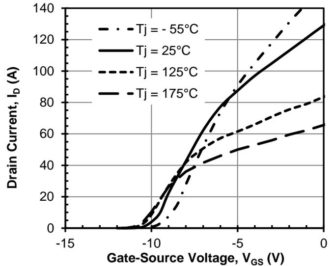
**Figure 6** Typical transfer characteristics at  $V_{DS} = 5V$
