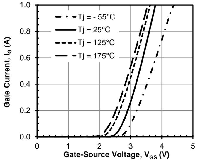
**Figure 14 Typical gate forward current at  $V_{DS} = 0V$**
