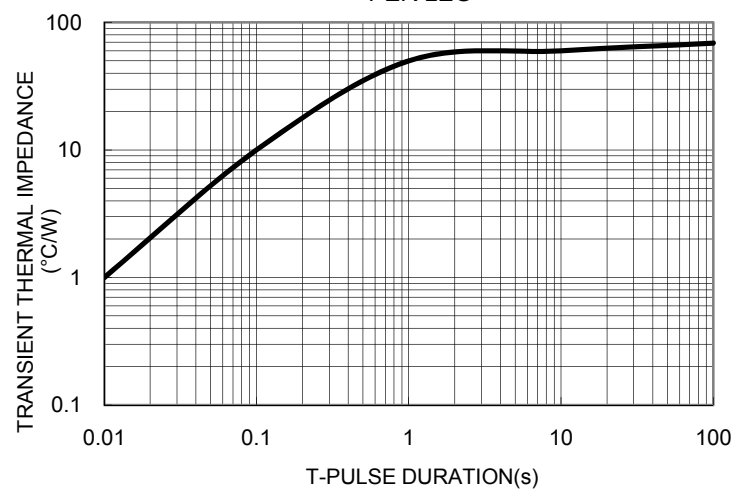
FIG. 6 TYPICAL TRANSIENT THERMAL IMPEDANCE PER LEG
