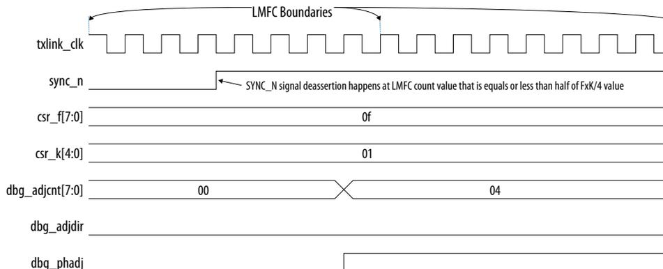
**Figure 16. Timing Diagram Example for Case 3**
