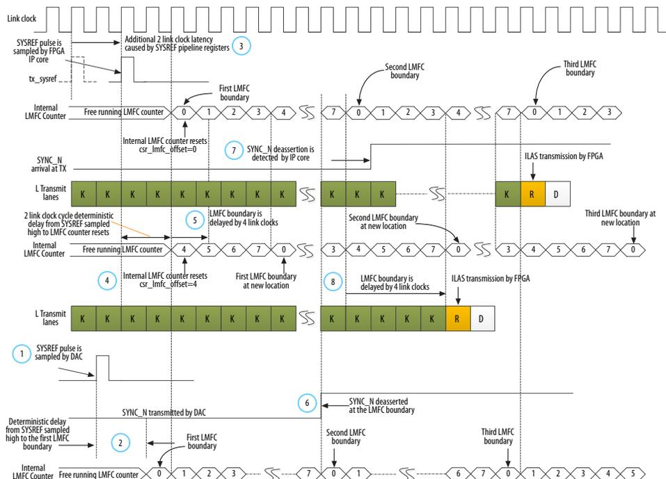
The `csr_lmfc_offset` field provides a convenient way to achieve deterministic latency and potentially optimizing the IP core latency. There are other ways that you can achieve deterministic latency by using the features available at the converters. Consult the converter manufacturer for details of these features.
