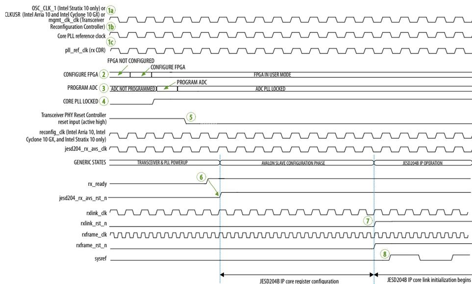
The recommended ADC – FPGA subsystem bring-up sequence:
