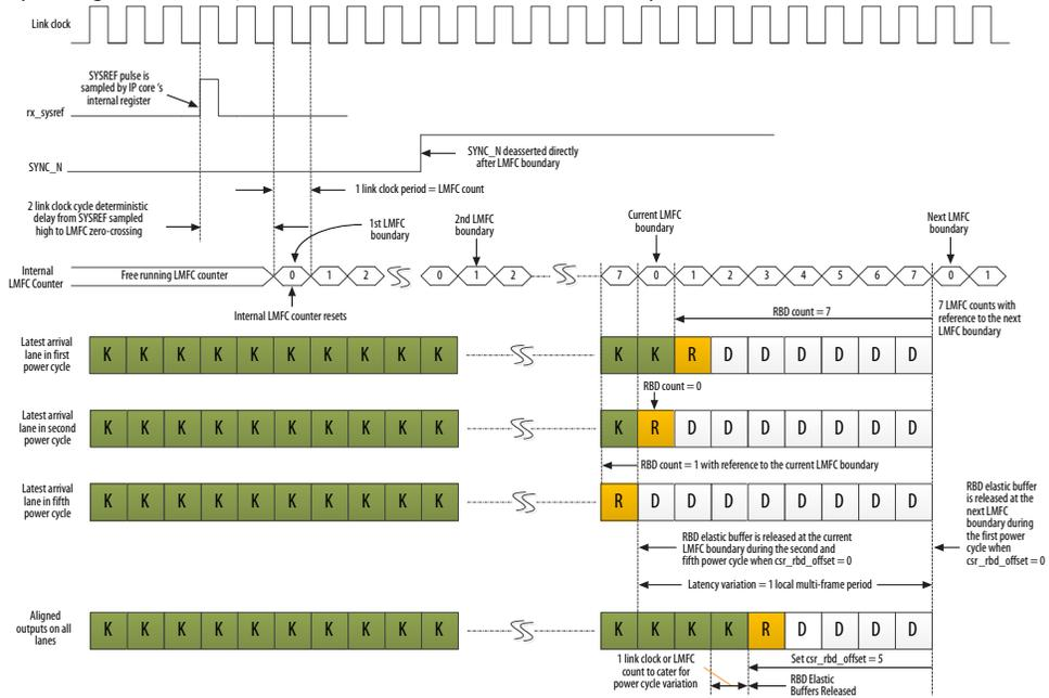
In the example above, lane deskew error happens if the sum of the difference of /R/ character's LMFC count in the earliest arrival lane to the latest arrival lane, and the number of LMFC count up to the release of RBD elastic buffer exceeds the RBD elastic buffer size. If this is the root cause of lane deskew error, setting RBD offset is one of the techniques to overcome this issue. Not every RBD offset value is legal. Figure below illustrates the technique to decide the legal RBD offset value.
