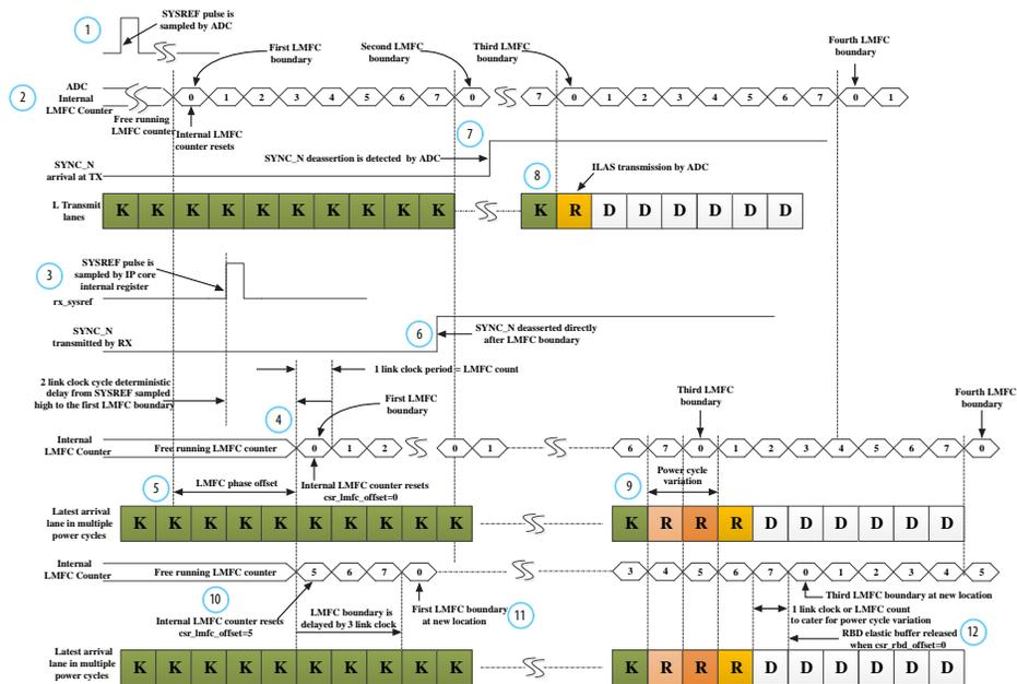
You should set a safe LMFC offset value to ensure deterministic latency from one power cycle to another power cycle. In [Figure 30](#) on page 155, the illegal `csr_lmfc_offset` values of 1, 2, and 3 causes lane de-skew error because the RBD buffer size has exceeded.
