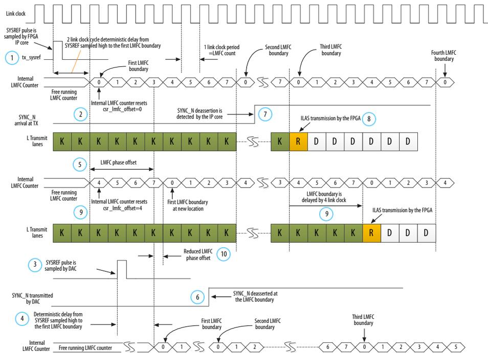
Alternative to tuning RBD offset at the DAC, adjusting TX LMFC offset in the FPGA helps you to achieve deterministic latency. You should perform multiple power cycles and read the RBD counts at the DAC to determine whether deterministic latency is achieved and RBD elastic buffer size has not exceeded.
