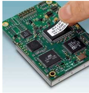
Stick-on device marking, removable, for printing with THERMOMARK ROLL... EML-RM... Page 286
