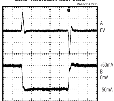
400ns/div A: OUTPUT VOLTAGE, 1V/div, AC-COUPLED B: OUTPUT CURRENT, 50mA/div
