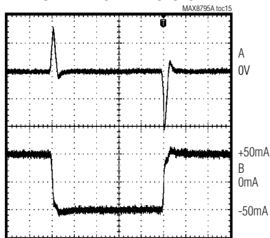
400ns/div A: OUTPUT VOLTAGE, 1V/div, AC-COUPLED B: OUTPUT CURRENT, 50mA/div
