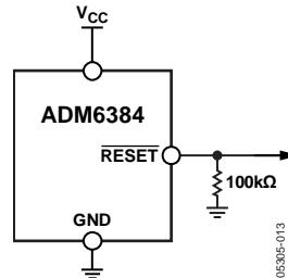
Figure 13. Ensuring Reset Valid to  $V_{CC} = 0$  V
