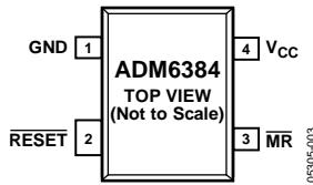
Figure 3. Pin Configuration
