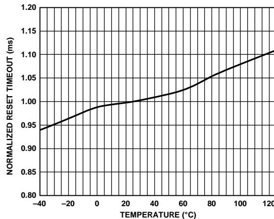
Figure 5. Normalized Reset Timeout Period vs. Temperature
