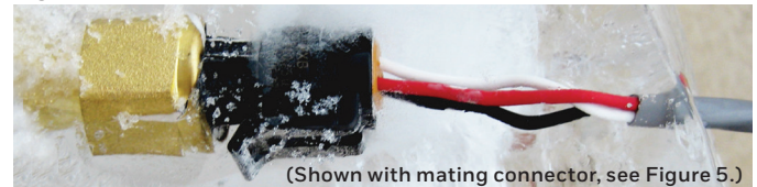
Figure 2. PX3 Series External Freeze/Thaw Resistance
