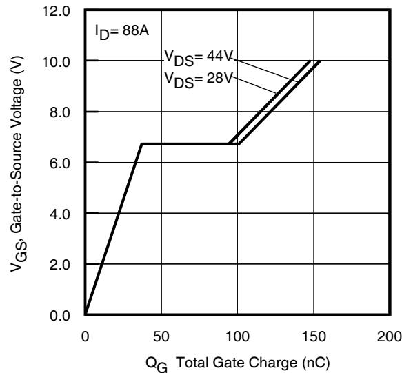
**Fig 6.** Typical Gate Charge vs.
