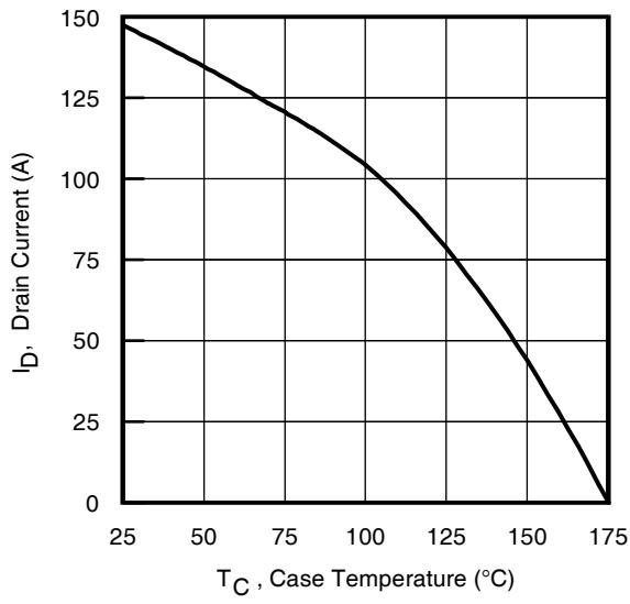
**Fig 9.** Maximum Drain Current vs.
