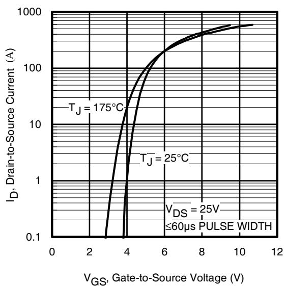
**Fig 3.** Typical Transfer Characteristics
