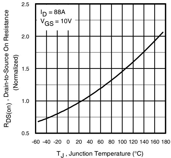
**Fig 10.** Normalized On-Resistance
