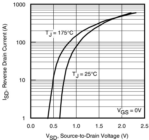
**Fig 7.** Typical Source-Drain Diode
