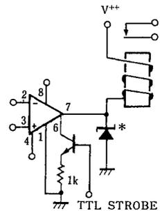
\*Absorbs inductive kickback of relay and protects IC from severe voltage.
