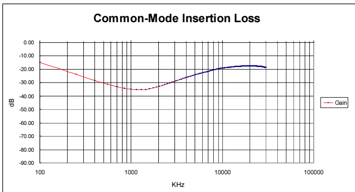
Typical Common-mode Loss for FM30R100P
