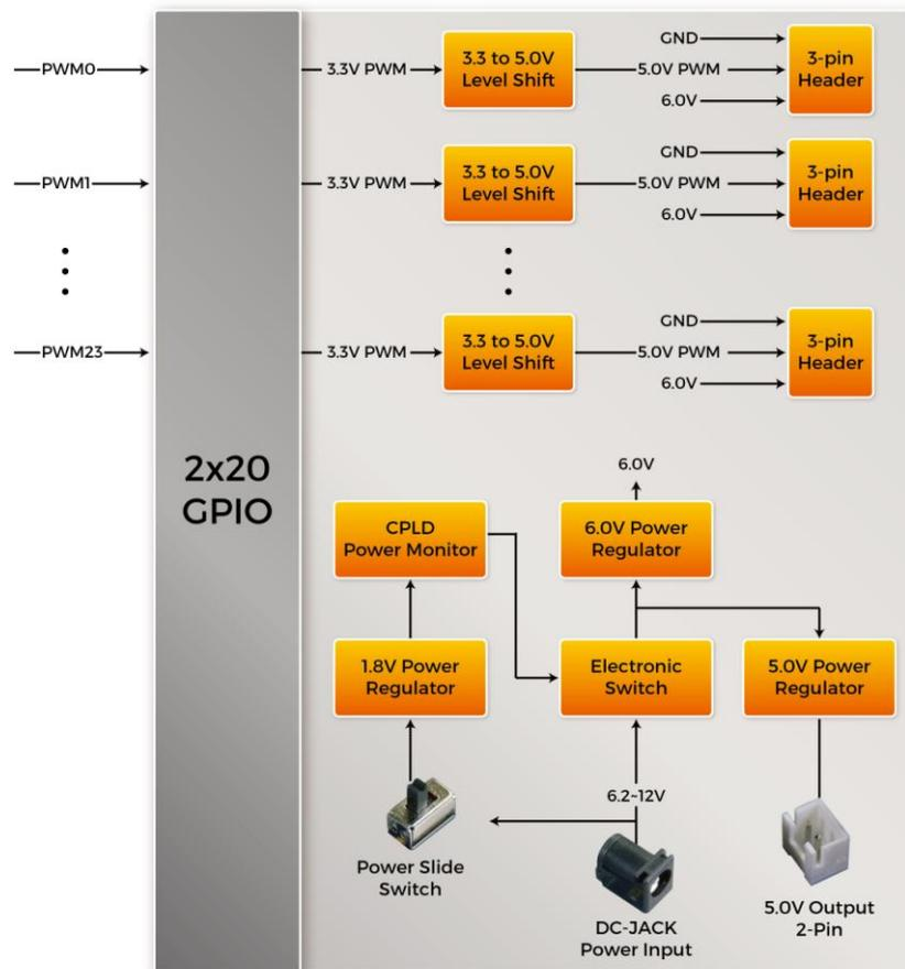
Figure 2-2 Block Diagram of Servo Motor Card
