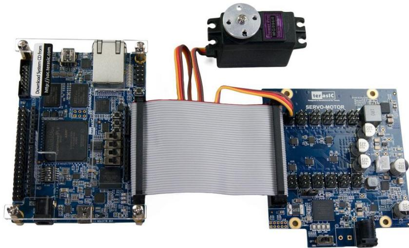
**Figure 1-5 Connect the Servo Motor and Motor Card to DE0-Nano-SoC**
