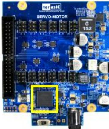
**Figure 2-12 CPLD for Power Monitor**
