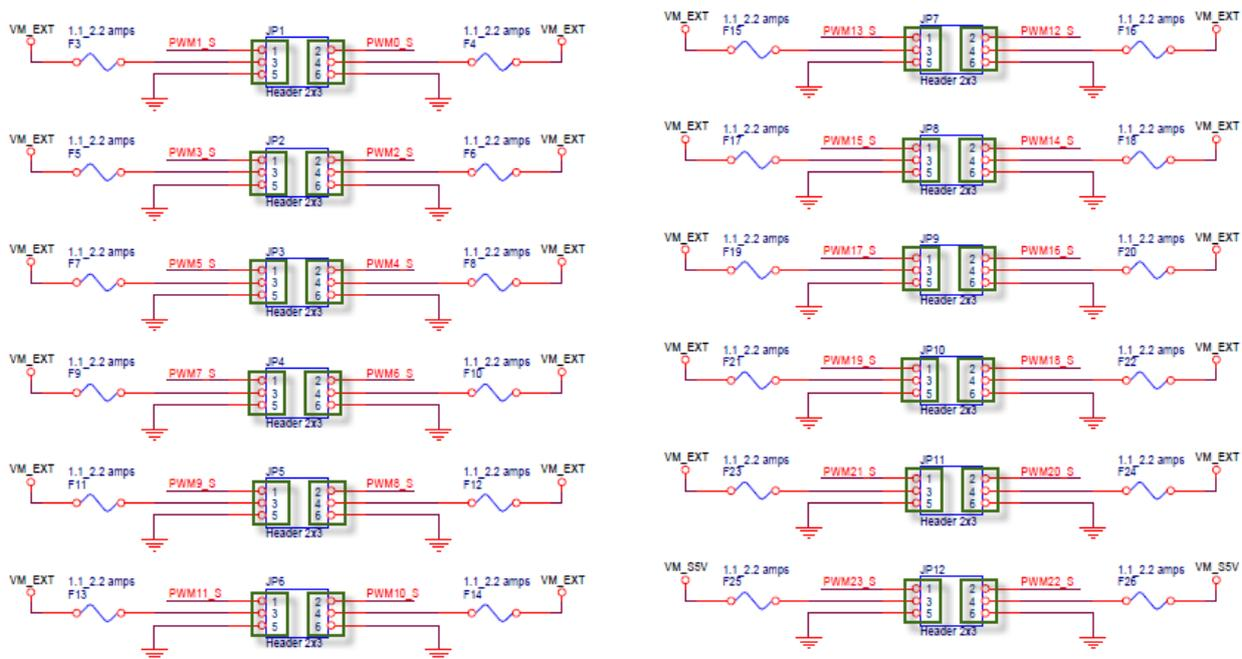
**Figure 2-10 24 1x3 header for 24 servo motors**
