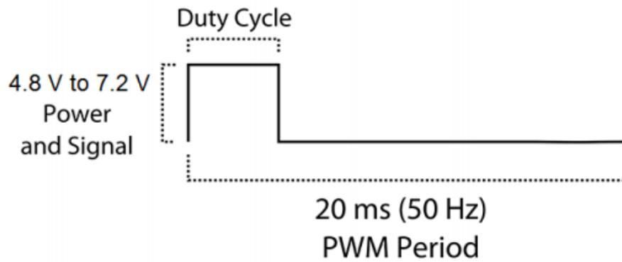
**Figure 2-14 PWM Duty Cycle and Period**
