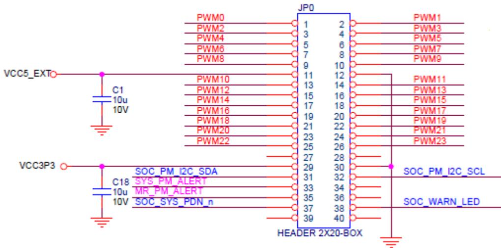
**Figure 2-6 2x20 GPIO Pinout**
