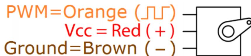
**Figure 2-13 Three wires of server motor connector**
