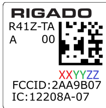
Figure 9 - R41Z MAC Address on Label
